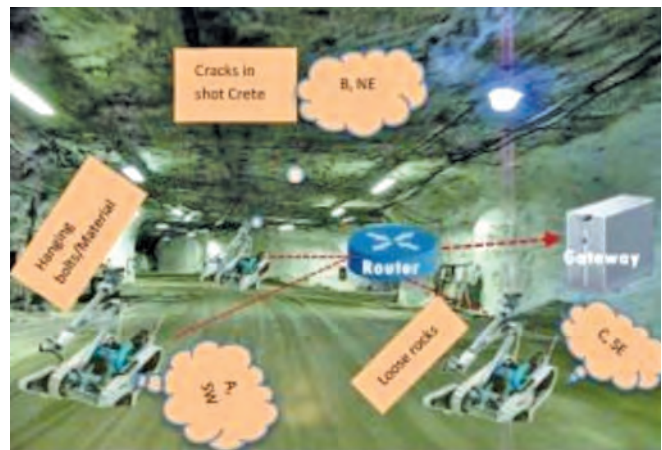
Fig.9 Robots inspecting for rock falls in an underground mine while communicating [23]
