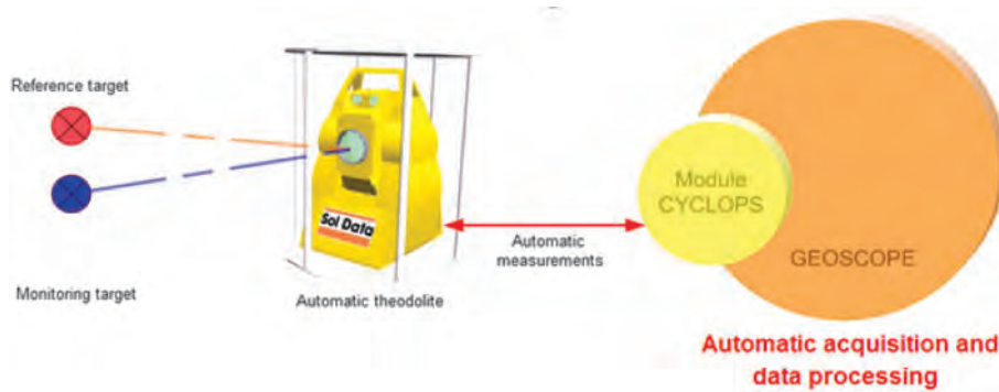
Fig.8 Principle of operation of slope stability real time monitoring by Cyclops (Source: www.soldatagroup.com)
