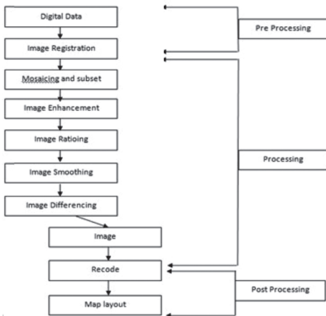
Fig.2 Schematic representation of data row for land use change detection studies in JCF
