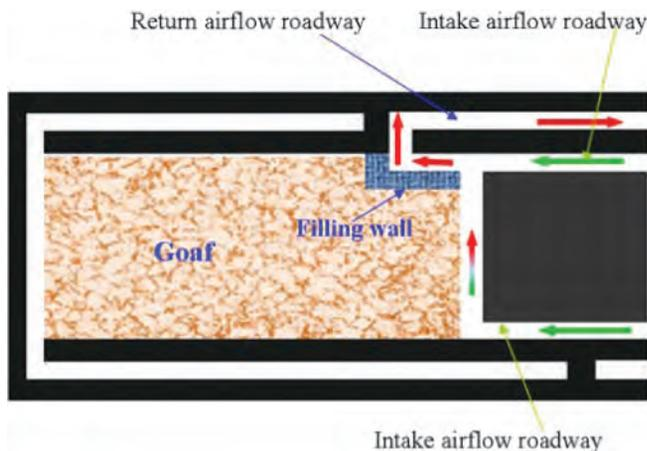
Fig.2 Layout of 42207 workface
