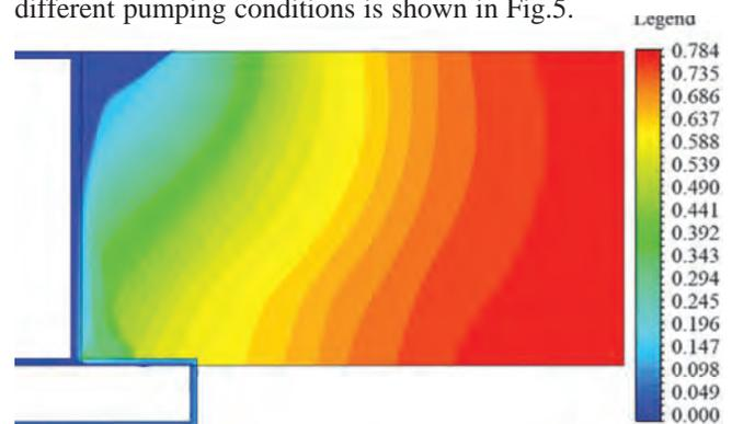
(a) The mixed volume for gas drainage of drainage pipe is 100 m<sup>3</sup>/min
