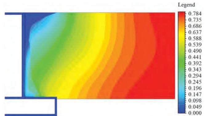
Fig.7 Gas concentration distribution in the goaf with 2m away from the floor of coal seam by multiple drainage pipes
