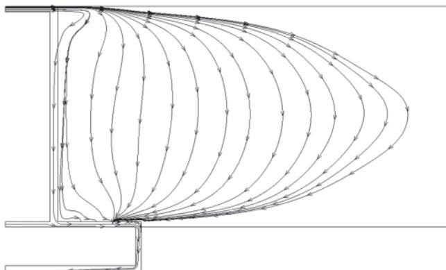
Fig.6 Flow field with 2m away from the floor of coal seam by multiple drainage pipes
