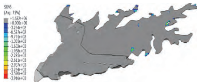
Fig.5 Liquefied region of 4s (unsaturated region is translucent)
