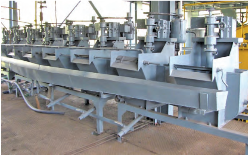
Fig.3 Pilot scale flotation cells (400 kg/hr capacity)
