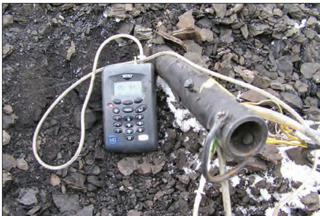
Fig. 3: Measurement of CO_2 using the infrared analyser Geotech G110
