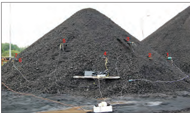
Fig. 2: Location of probes in the coal stockpile (photo VUHU Most)
