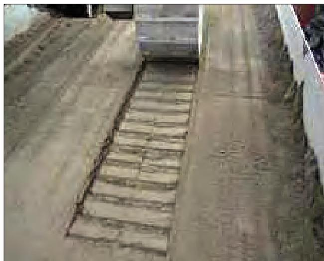
Fig. 3. The rutting in lunar soil simulants
