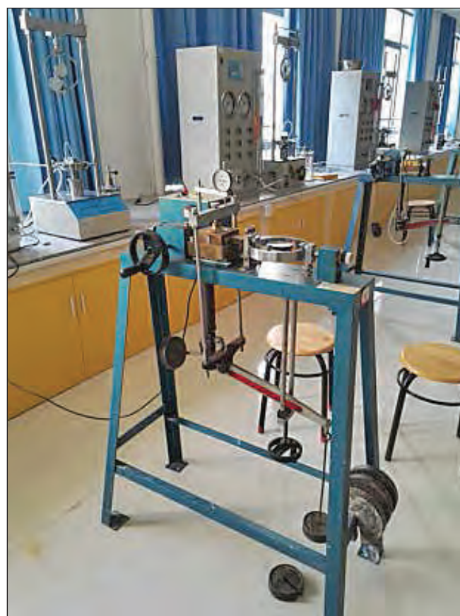
Fig. 2: Overview of direct shear test system
