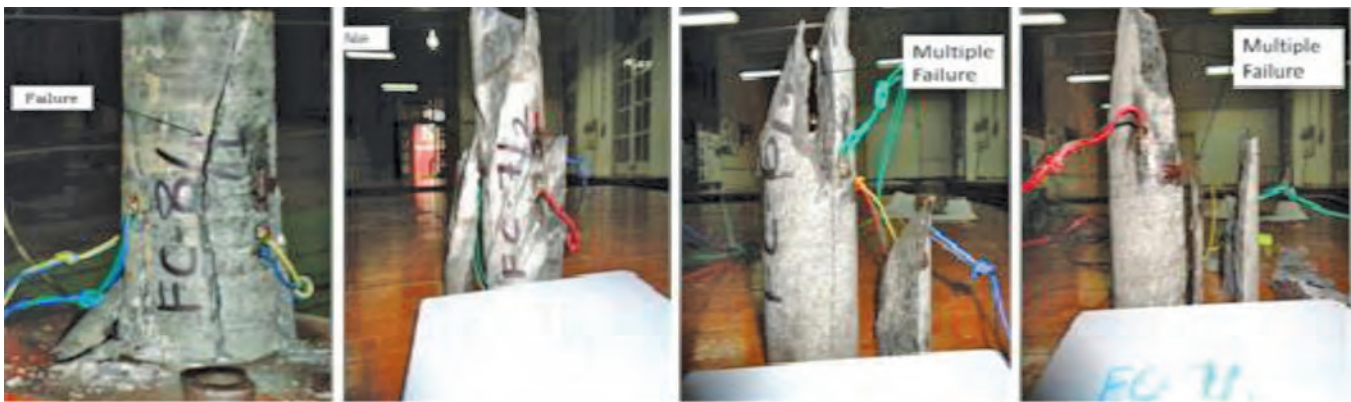
Fig.5(a) Failure occurred during UCS testing in footwall sample
