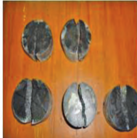
(f) Footwall sample showing failure.
