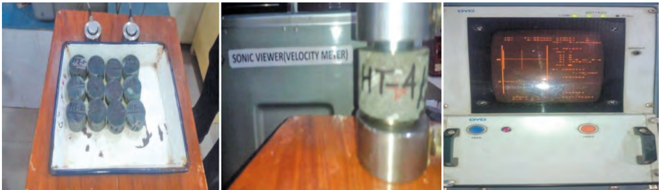
(a) Sample with transducer (b) Sonic viewer machine (c) Graph on the machine
