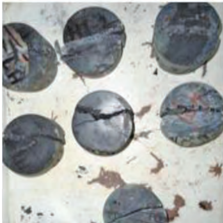
(e) Hanging wall samples showing failure.
