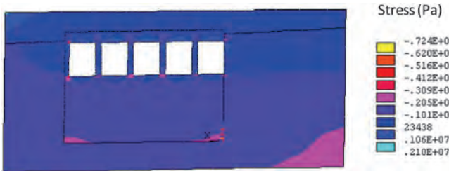
Fig.8 Minor principal stresses of vertical section
