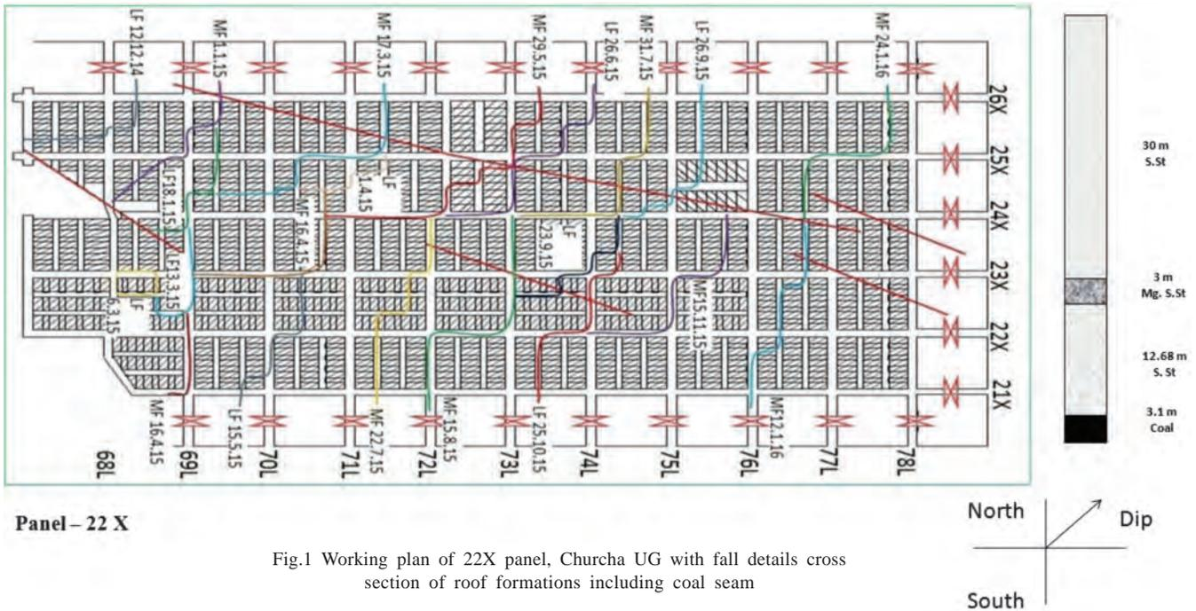
Fig.1 Working plan of 22X panel, Churcha UG with fall details cross section of roof formations including coal seam
