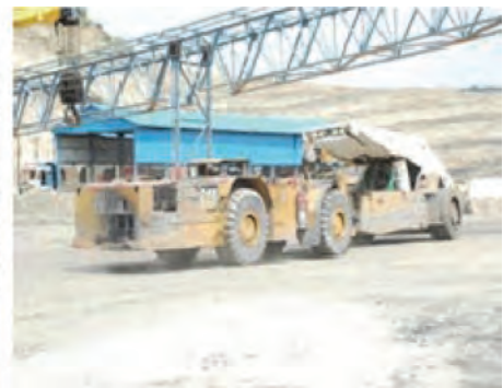
Fig.8(a) and (b) Brake testing on RAMP & Transportation of PRS with diesel vehicle
