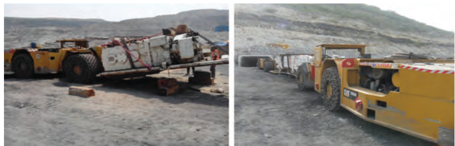
Fig.6 Transport of MG drive and shearer with SH660D
