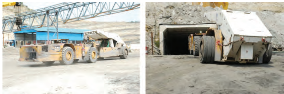
Fig.5 Transport of shield with SH150 shield trailer
