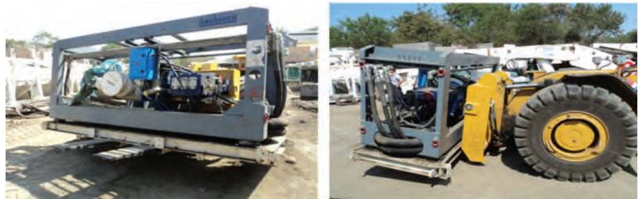
Fig.4 Transport of pump unit with CLT210
