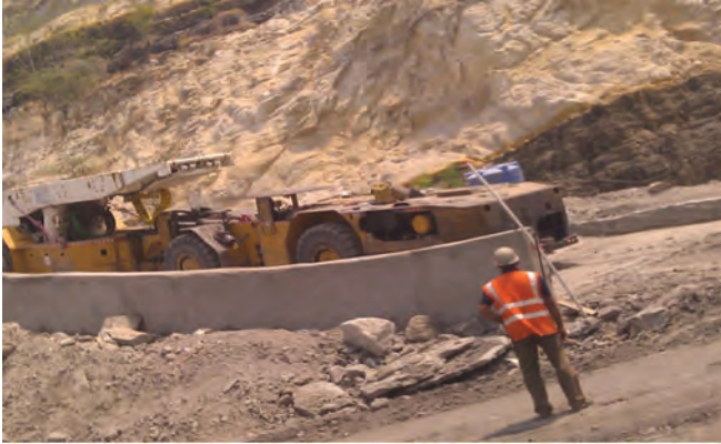
Fig.7 Testing of braking efficiency of diesel vehicles on test ramp
