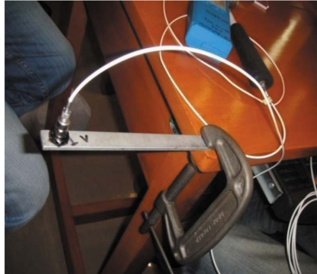
Figure 1. Damping test arrangement.
