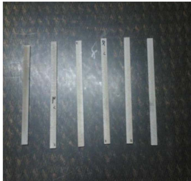
Figure 2. Damping test specimen.
