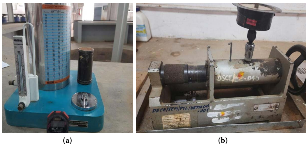
Figure 1. Equipment's used for testing properties of mould sand. (a) Permeability test (b) Compression test.
