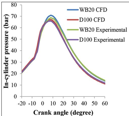
Figure 8: Comparison of experimental and simulated in-cylinder pressure
