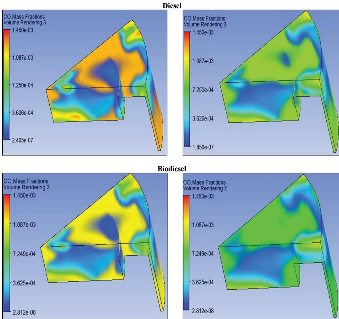
Figure 7: CO mass fraction for diesel and biodiesel fuels
