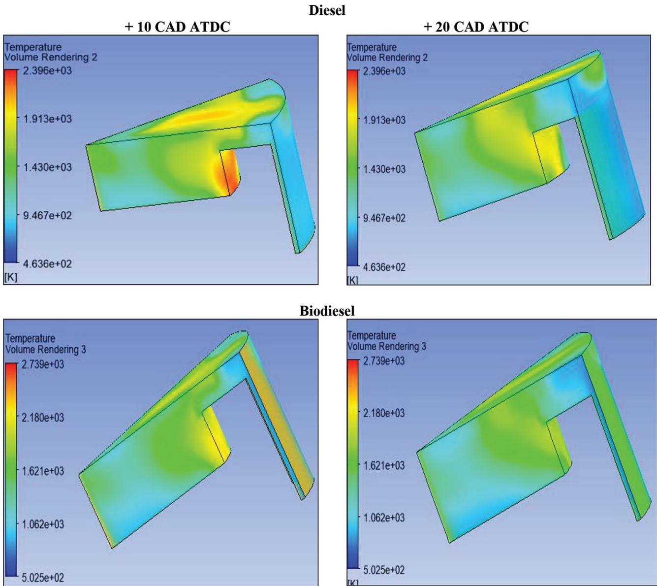
Figure 4: In-cylinder temperature of spatial plots for diesel and biodiesel.
