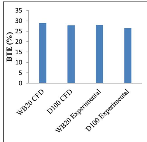
Figure 9: Comparison of experimental and simulated BTE
