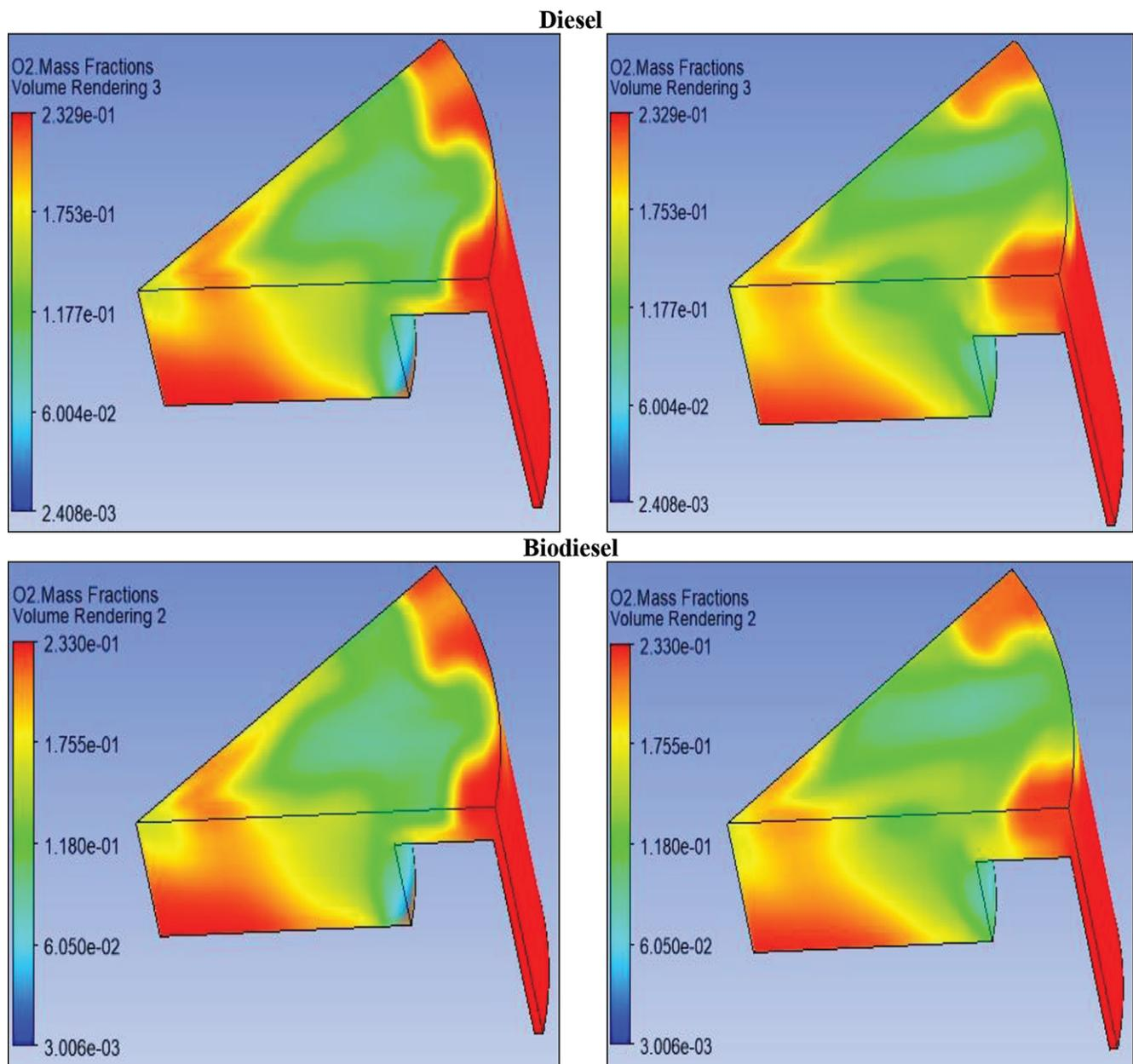
Figure 5: O<sub>2</sub> mass fraction for diesel and biodiesel fuels
