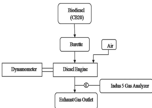
Figure 2: Flow map of the engine tests
