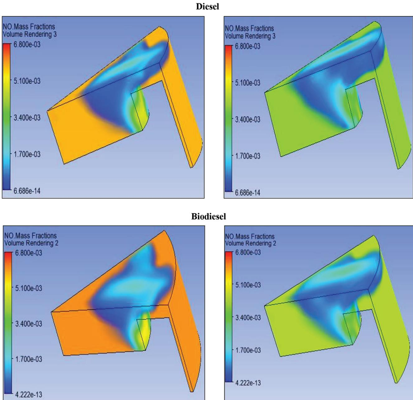
Figure 6: NO mass fraction for diesel and biodiesel fuels
