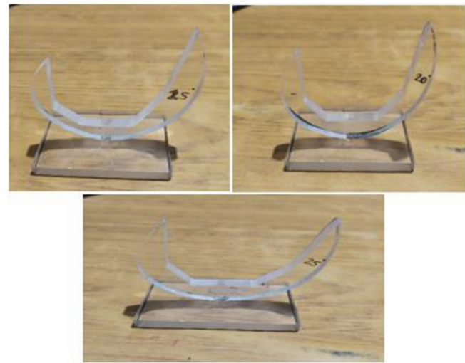
Figure 2: Photoelastic models for 40mm radius and different angles
