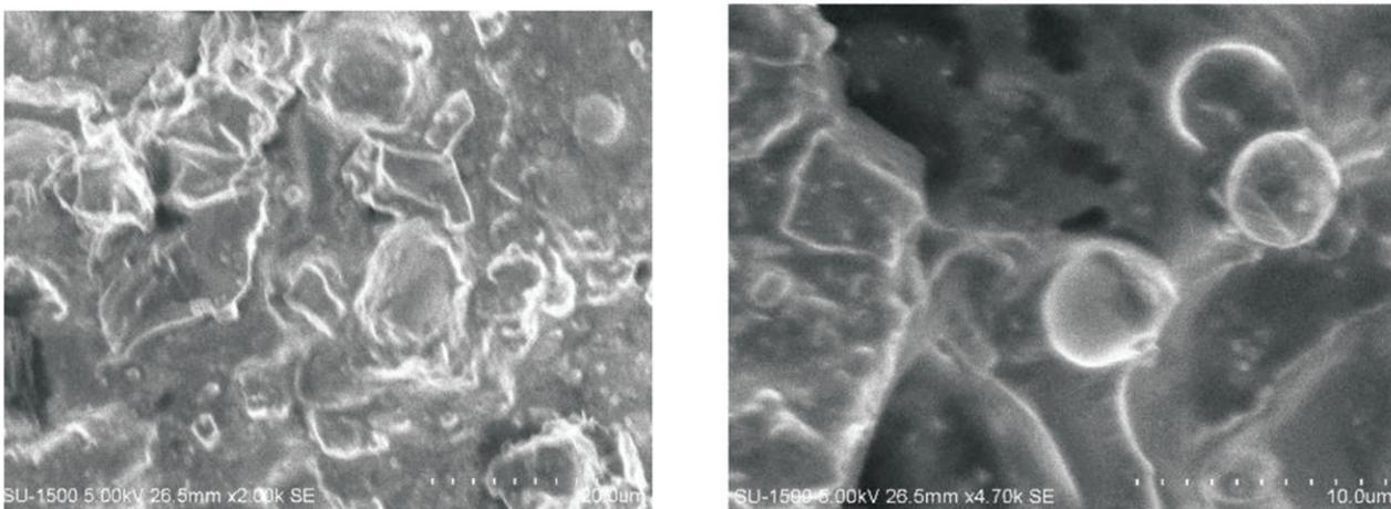
Figure 10: SEM images of C-FRP coated with WCC
