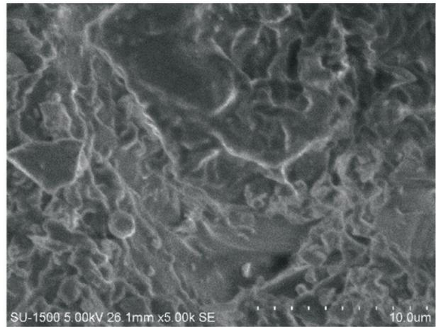
**Figure 5:** SEM images of Bamboo FRP coated with Cr<sub>2</sub>O<sub>3</sub> (Ceramic Coating)
