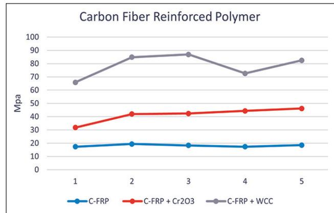
Figure 13: Microhardness of C-FRP with and without coating
