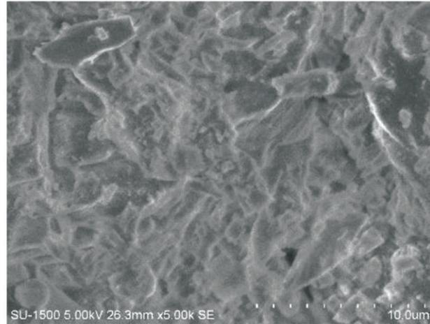
**Figure 6:** SEM images of SiC-FRP coated with Cr<sub>2</sub>O<sub>3</sub> (Ceramic Coating)
