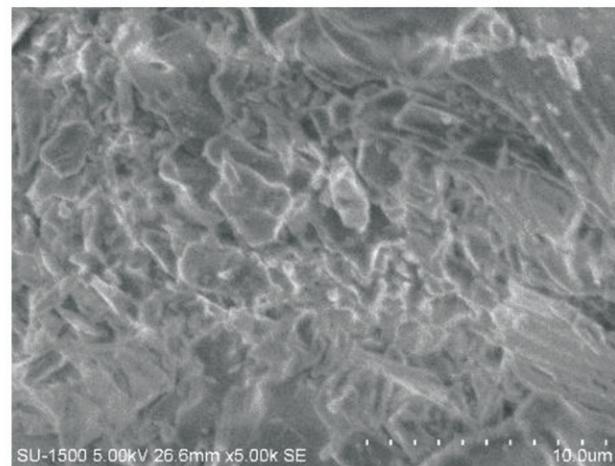
**Figure 7:** SEM images of C-FRP coated with Cr<sub>2</sub>O<sub>3</sub> (Ceramic Coating)
