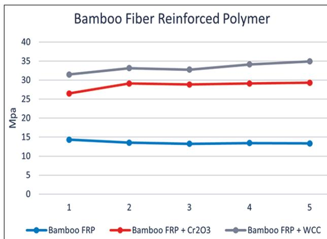
Figure 11: Microhardness of Bamboo FRP with and without coating
