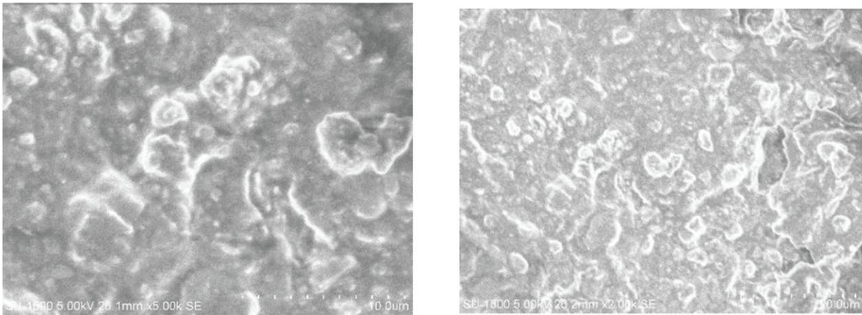
Figure 9: SEM images of SiC-FRP coated with WCC
