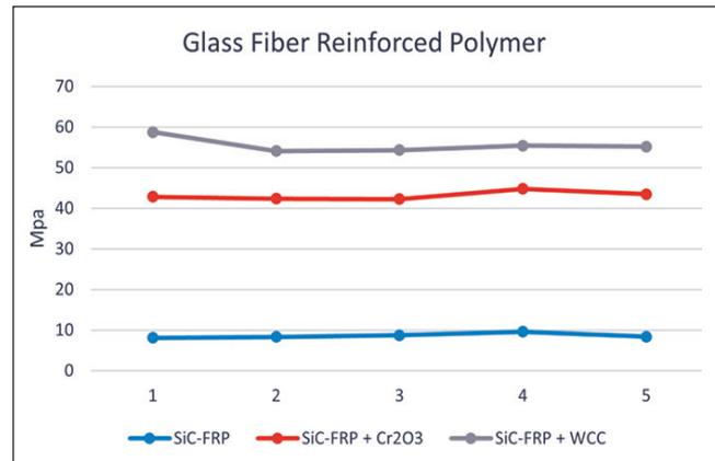
Figure 12: Microhardness of SiC-FRP with and without coating
