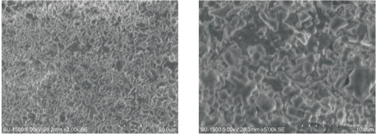
Figure 8: SEM images of Bamboo FRP coated with WCC
