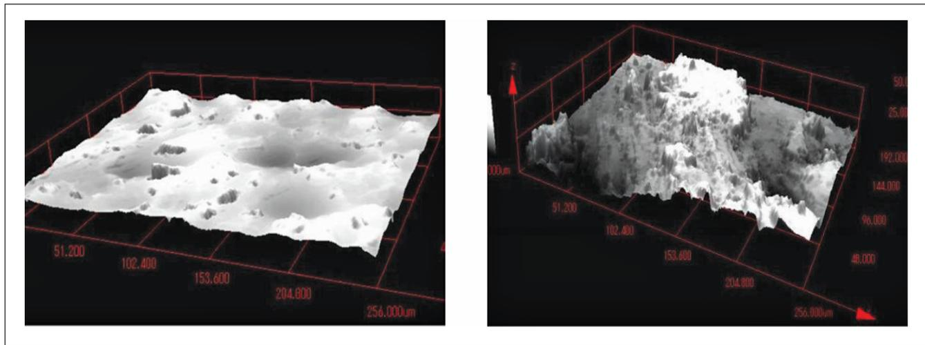
**Figure 3:** Laser optical Microscopy of the surface profile of (a) Untreated C-FRP and (b) Mechanically treated C-FRP
