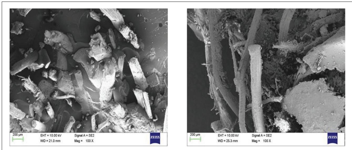
**Figure 4:** SEM micrographs of Bamboo FRP after conductive coating
