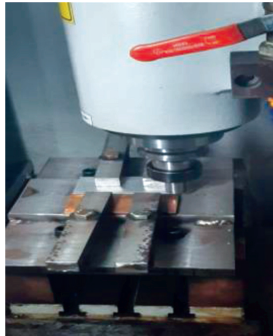
Figure 4: Test set up to conduct FSW of Al-Cu joint
