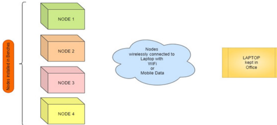
Figure 3. Implementation of Wireless Sensor Network.
