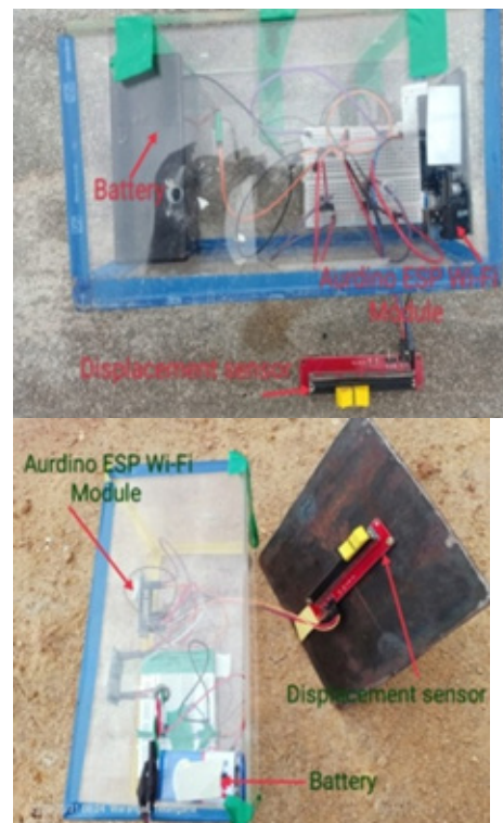
Figure 10. Different displacement sensor nodes were prepared for installation.
