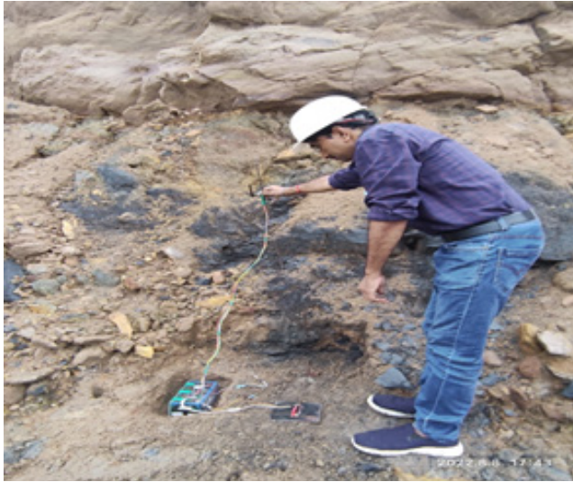
Figure 15. Monitoring of slope deformation using wireless sensors in the field.
