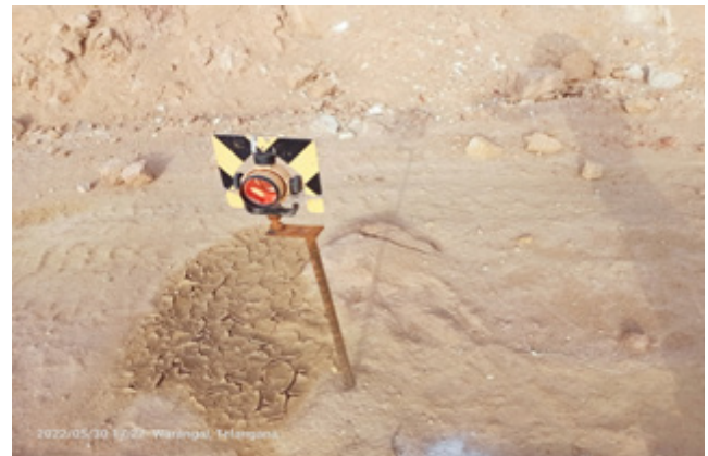
Figure 16. Slope monitoring with the total station by the mine authorities.
