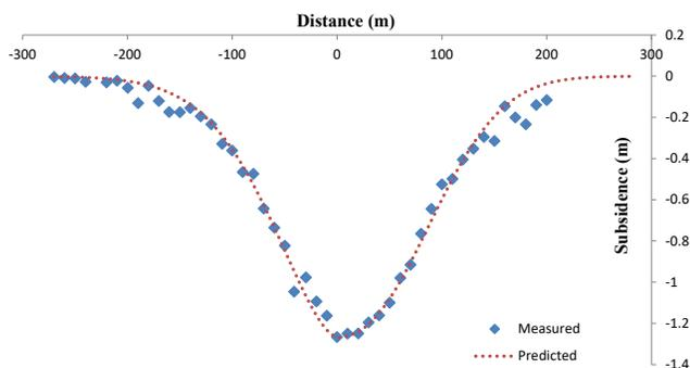
**Figure 12.** Measured and predicted surface subsidence over longwall panel no.1.
