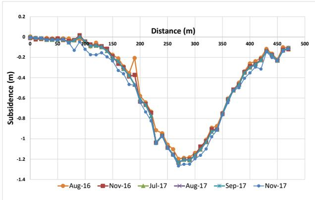
**Figure 7.** Subsidence profile along the path ‘S’ of Longwall panel no.1.
