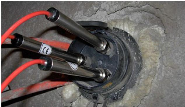
**Figure 3.** Multipoint borehole extensometer.
