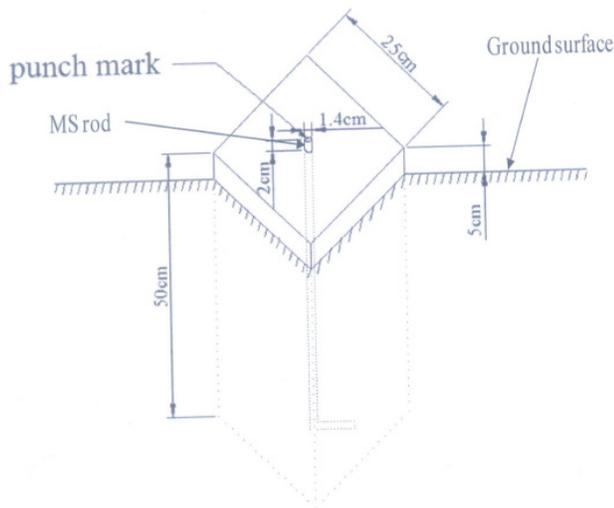
Figure 5. Design of subsidence pillar.
