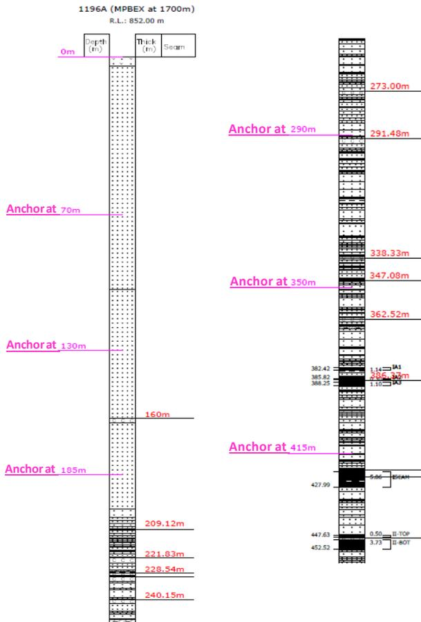
**Figure 8.** Borehole section showing the anchoring points of MPBX 1700.
