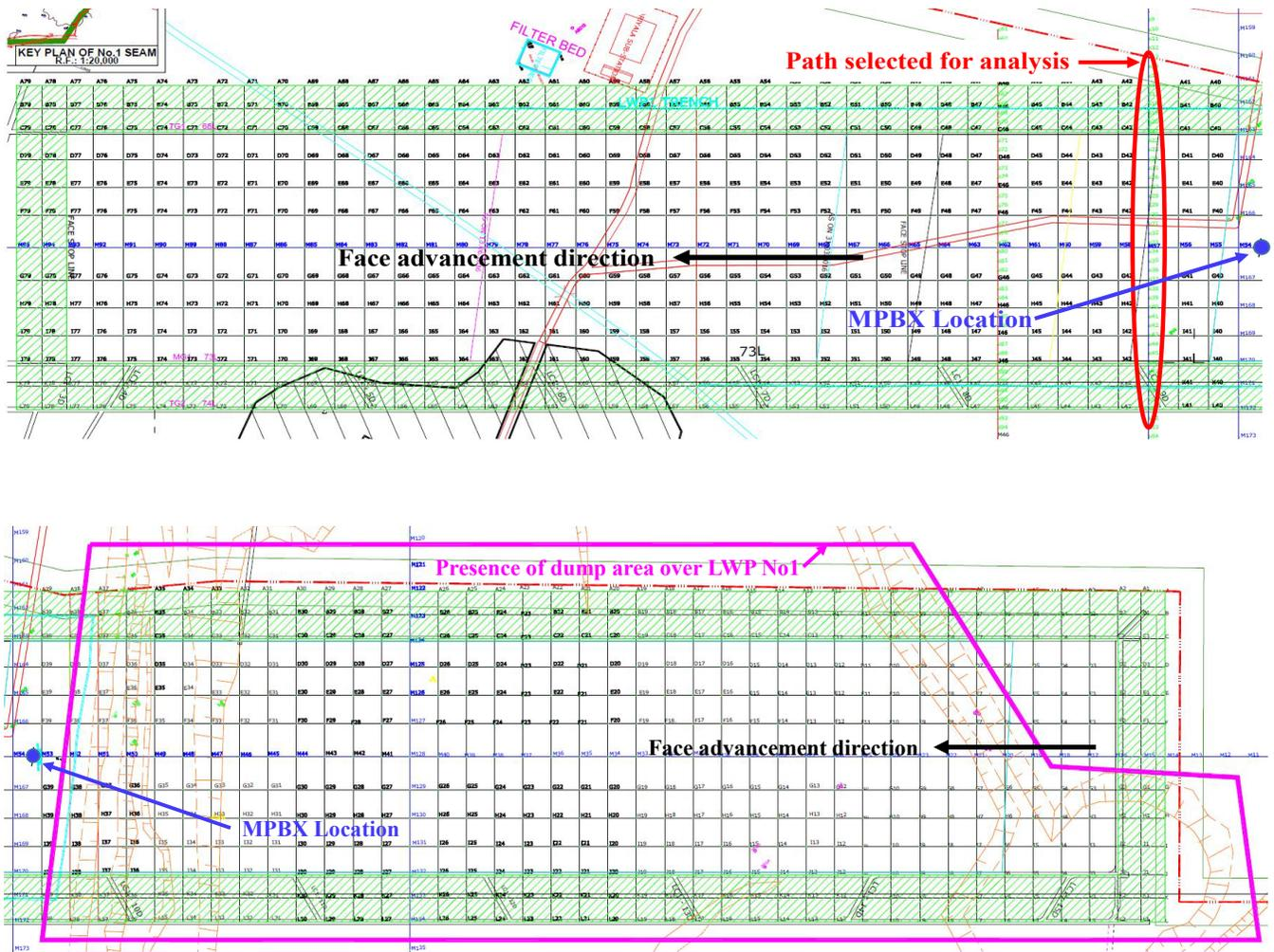
Figure 4. Surface monitoring plan of longwall panel no.1 at Adriyala.
