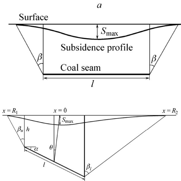
**Figure 10.** Profile of subsidence in (a) horizontal and (b) inclined seams.
