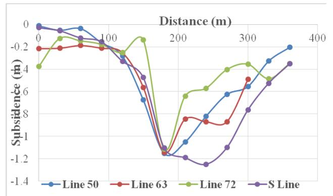
Figure 6. Subsidence profile at different
