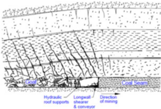
**Figure 1.** Schematic diagram showing the Longwall Face (Mine Subsidence Engineering Consultants, 2007).
