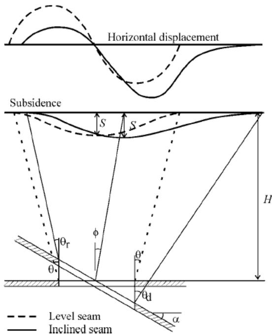
**Figure 2.** Nature of subsidence troughs caused by level and inclined seam extractions.
