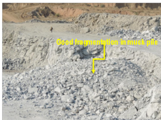
Figure 12. Good fragmentation in muck pile (V-type firing pattern).
