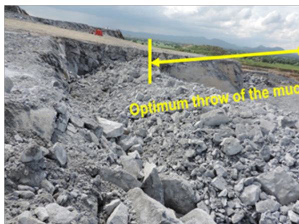
Figure 15. Optimum throw of muck pile (V-type firing pattern).
