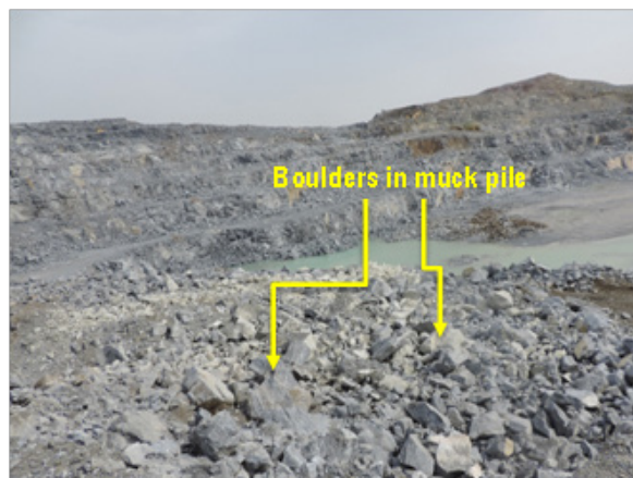
Figure 11. Boulder in muck pile (Diagonal firing pattern, LHS).
