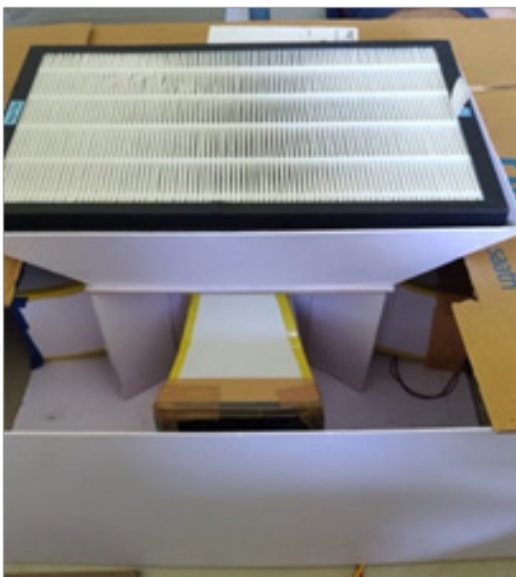
Figure 5. Construction of filter chamber.
