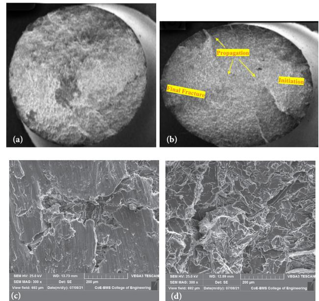
**Figure 13.** (a) A356-Hematite 9wt % of composite without copper chill, (b) A356-Hematite 9wt % of composite with copper chill, (c) Crack In A356-Hematite 9wt % of composite without copper chill, (d) crack In A356-Hematite 9wt % of composite with copper chill.
