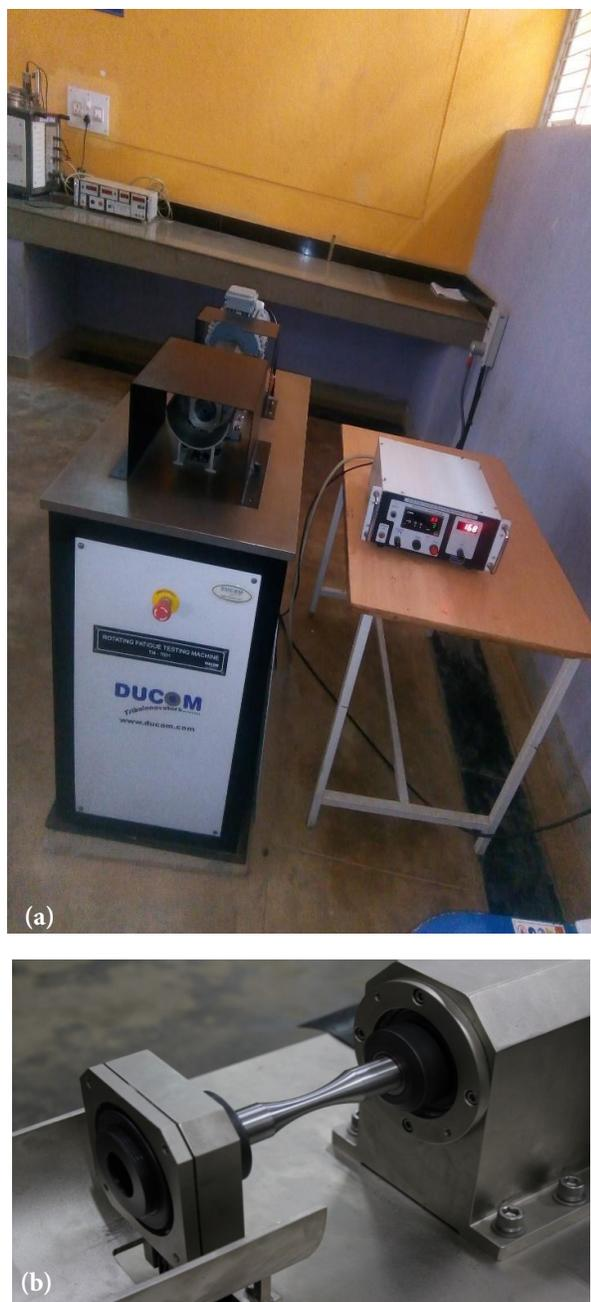
**Figure 6.** (a) Fatigue Testing machine, (b) Fatigue Testing machine with specimen attachment.
