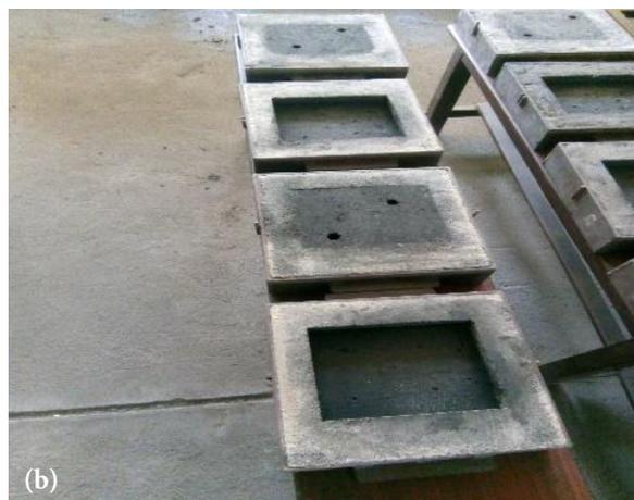
**Figure 3.** (a) Mould with Copper chill, (b) Mould without Copper chill.
