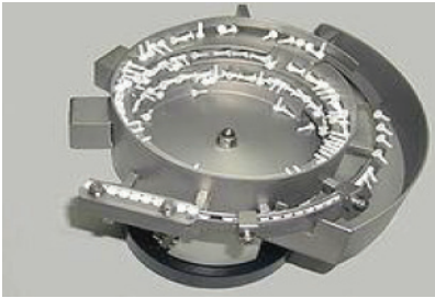
Figure 1: Vibratory Feeder Bowl Outer Diameter 300mm Input Power 220v 50Hz Ac
