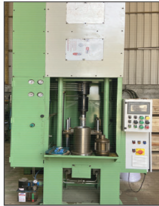
Figure 4: VM 800mm vertical honing machine
