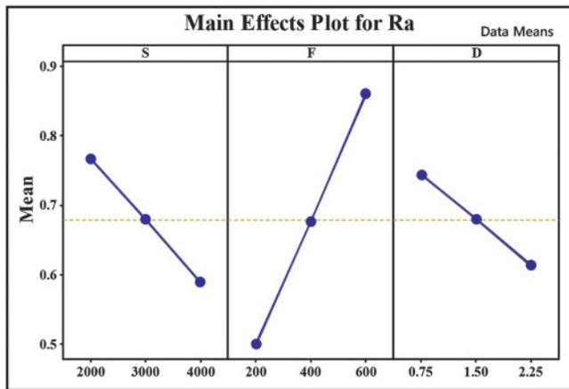
Figure 6: Main effects plot for average surface roughness
