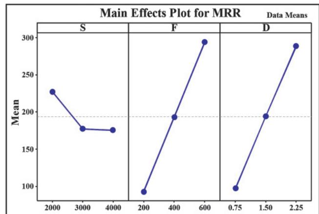
Figure 8: Main effects plot for material removal rate
