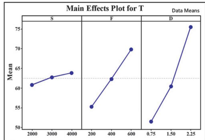
Figure 7: Main effects plot for cutting tool tip temperature rise
