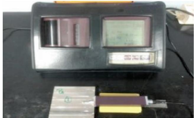
Figure 3: Surface roughness tester
