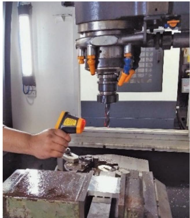
Figure 1: Cutting tool tip temperature measurement
