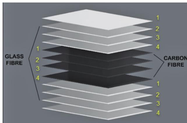
Figure 2: Stacking sequence of glass and carbon cloth
