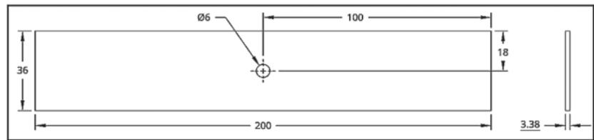
Figure 4: ASTM D5766 dimensions [14]
