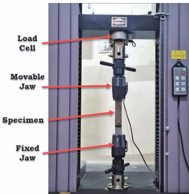
Figure 5: Wance UTM (50 kN capacity)
