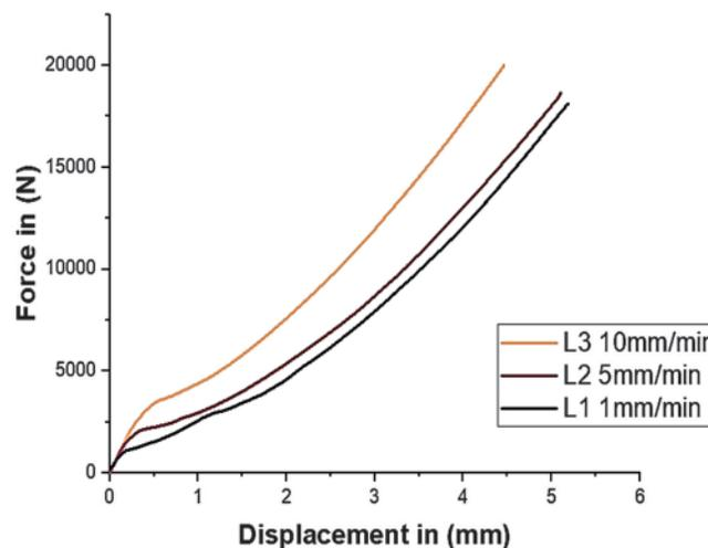
Figure 6: Load Vs displacement curves of hybrid glass and carbon composite
