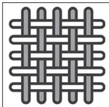
Figure 1: Plain weave pattern of individual glass and carbon fabric
