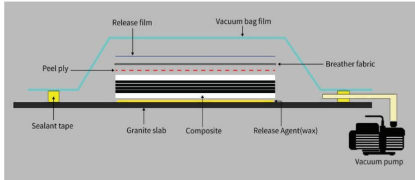
Figure 3: Vacuum bagging setup
