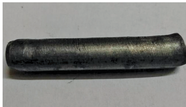
Figure 3: Homogenized AZ91 Mg alloy processed at 425°C
