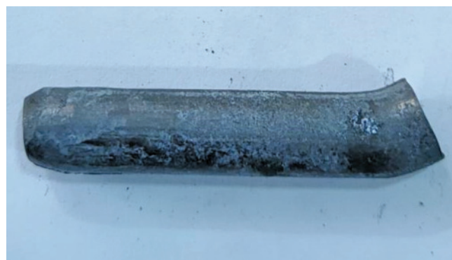
Figure 2: Non-homogenized AZ91 Mg alloy processed at 420°C
