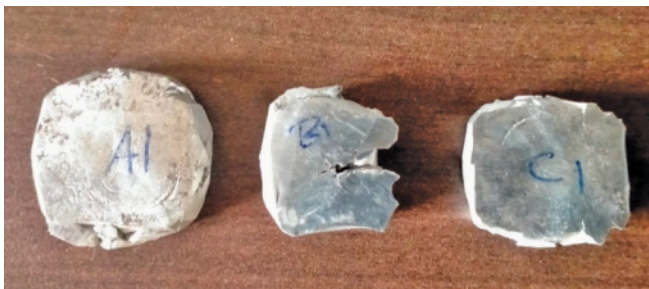
Figure 6: Specimen after Compression Test
