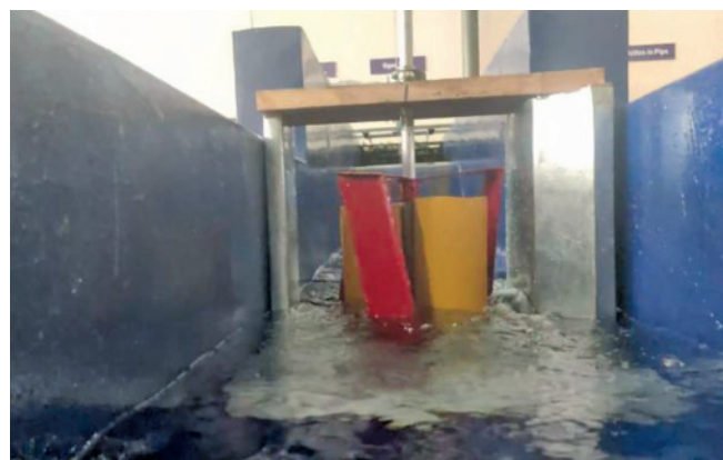
Figure 10: Placement of turbine in channel
