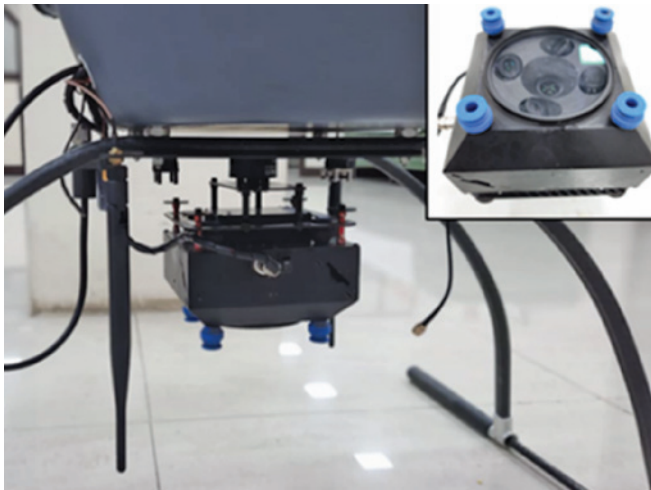
Figure 2: Drone mounted Sony 24 mp photogrammetric camera/sensor
