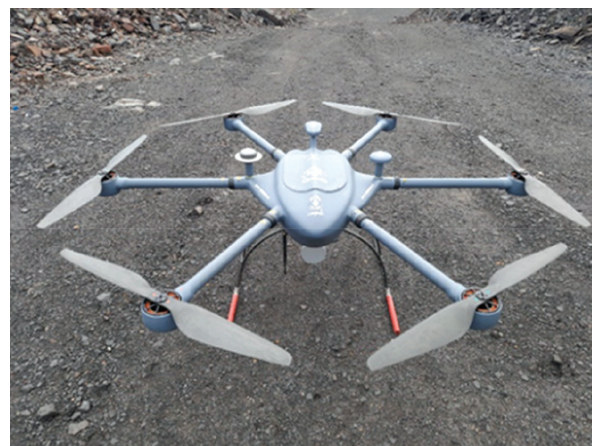
Figure 1: Co-axial Hexacopter Fitted with Velodyne Lidar
