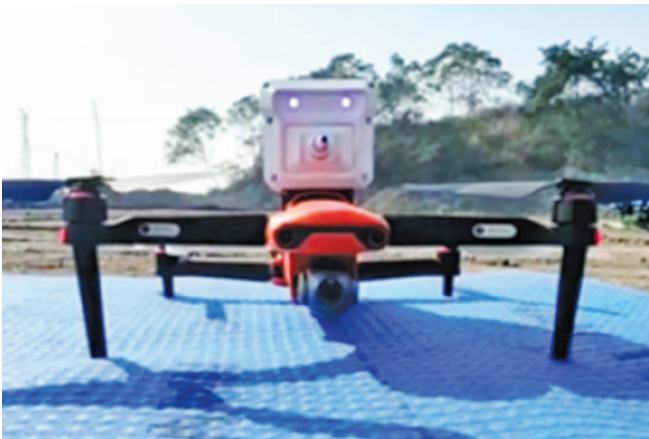
Figure 10: Drone fitted with gas detection module and PM • Concentration Distribution
