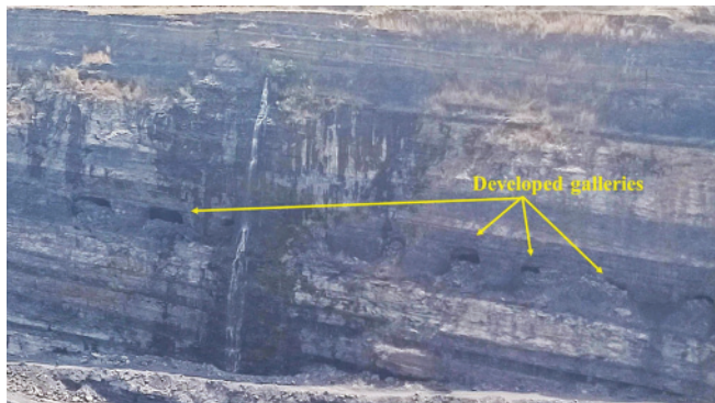
Figure 3(a): Old developed galleries are being seen in the opencast bench
