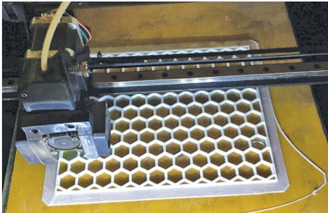
Figure 2: 3D-printing of honeycomb core with HYDRA-300
