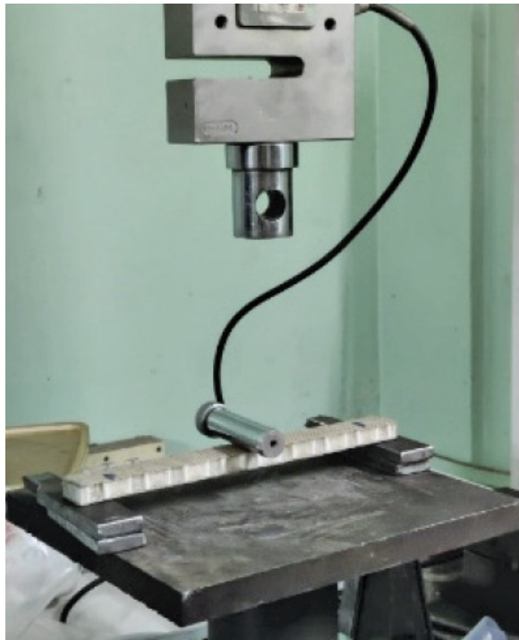
Figure 5: Experimental setup for flexural test
