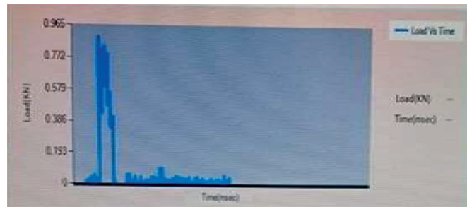
Figure 8: Impact Test Results for PLA materials
