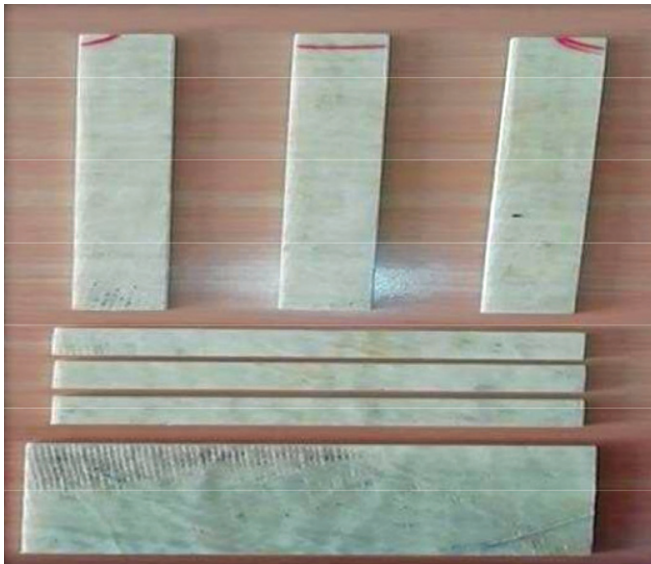
Figure 2: Composite material after water jet cutting
