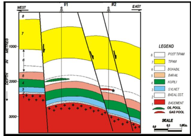
Figure 3. Geological cross-section along well #1 and well #2 of the field.
