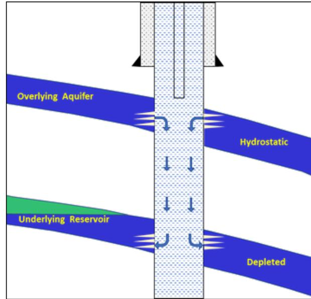
**Figure 13.** Schematic of a dump flooder.
