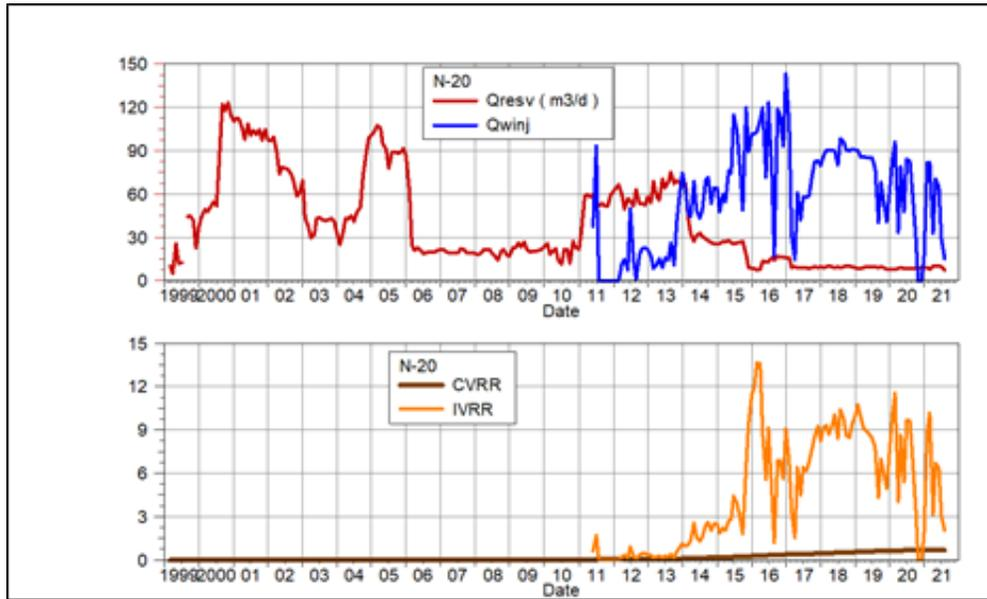
Figure 8. Voidage compensation profile in N-20 sand.
