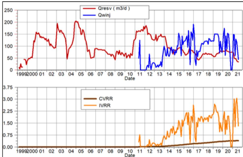
Figure 9. Voidage compensation profile in the field.
