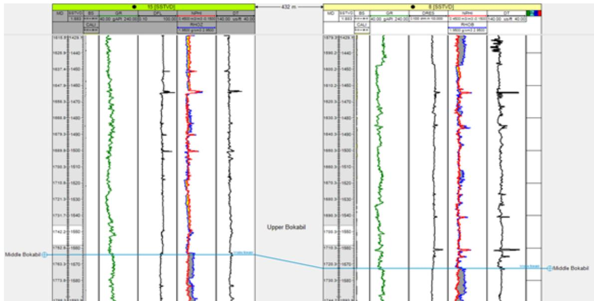
**Figure 14.** The upper Bokabil aquifer in the field serves as the source of water for dump flooding. (Shown on well logs of Injectors #8 and #15 above overlying Middle Bokabil).
