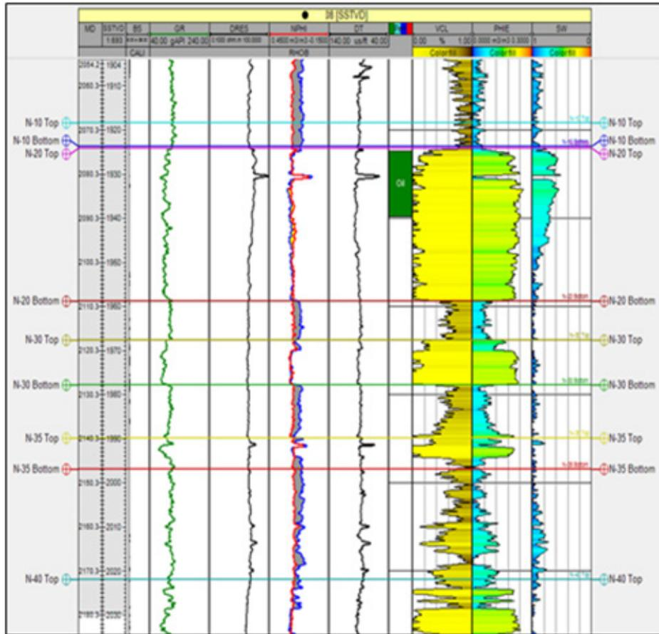
**Figure 11.** Rise in OWC in well #8 drilled in 2011.
