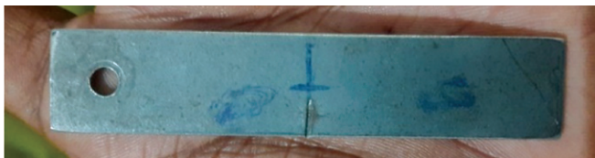
Figure 9: Crack length of 6mm
