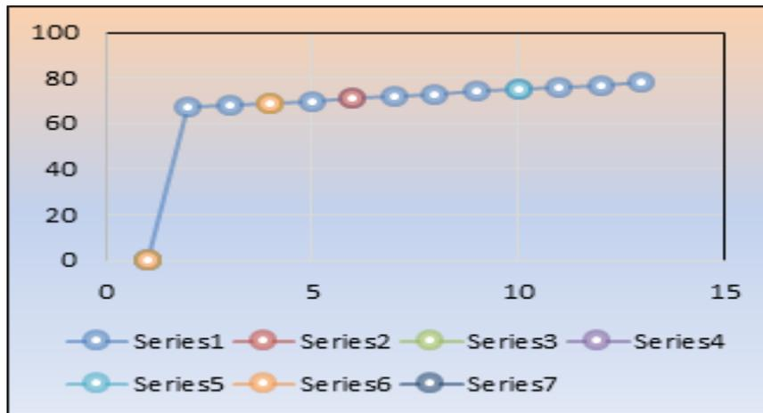
**Figure 14.** Vickers microhardness of the weldment.
