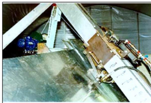
**Figure 16.** Portable FSW M/c on the ship parts welding.
