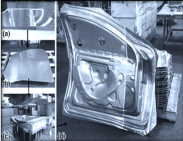
**Figure 17.** FSW of the car door.
