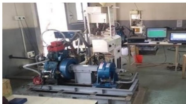
Figure 1. Computerized Variable Compression Ratio (VCR) gasoline engine.
