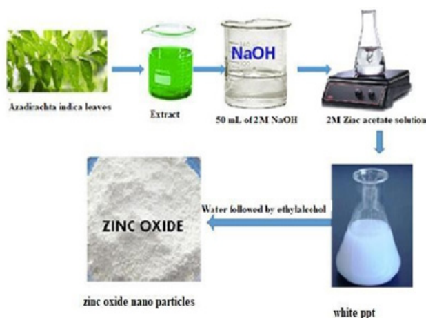
Figure 4. Zinc oxide nano particles: (Synthesis by using Azadirachta indica leaves).
