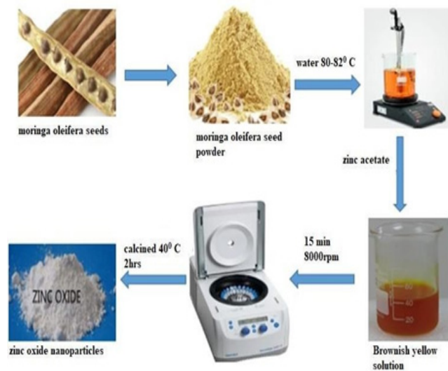
Figure 6. Green approach of zinc oxide nano particles: (by using Moringa oleifera seeds).
