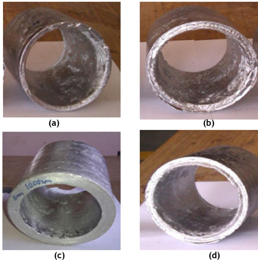
**Figure 2.** Casting of 8 mm thick Al-17Si rotated at the speeds of, (a) 600 rpm (b) 800 rpm (c) 1000 rpm (d) 1200 rpm.
