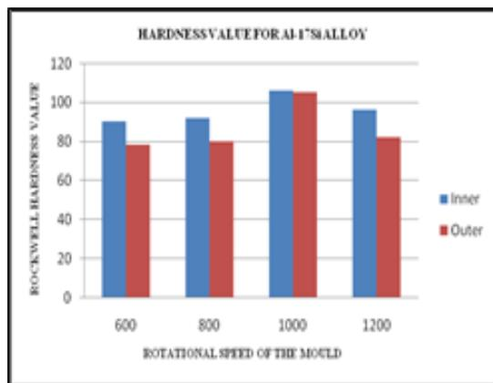
**Figure 6.** Hardness value v/s rotational speeds for 8 mm cast tubes of Al-17Si alloy.
