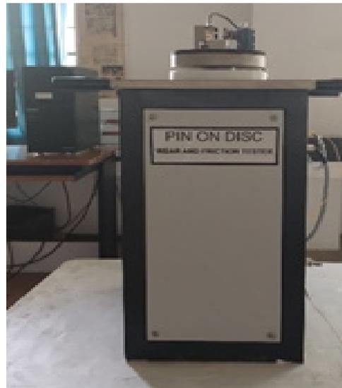
Figure 1. Wear and friction testing machine.
