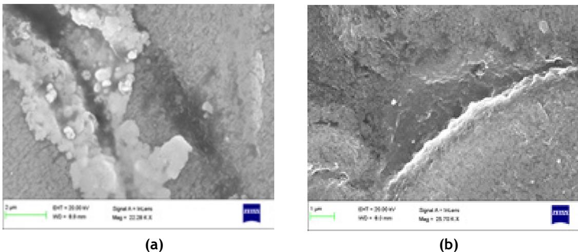
**Figure 8.** (a) Fractography images of 8 mm thick castings at 800 rpm. (b) Fractography images of 8 mm thick castings at 1000 rpm.
