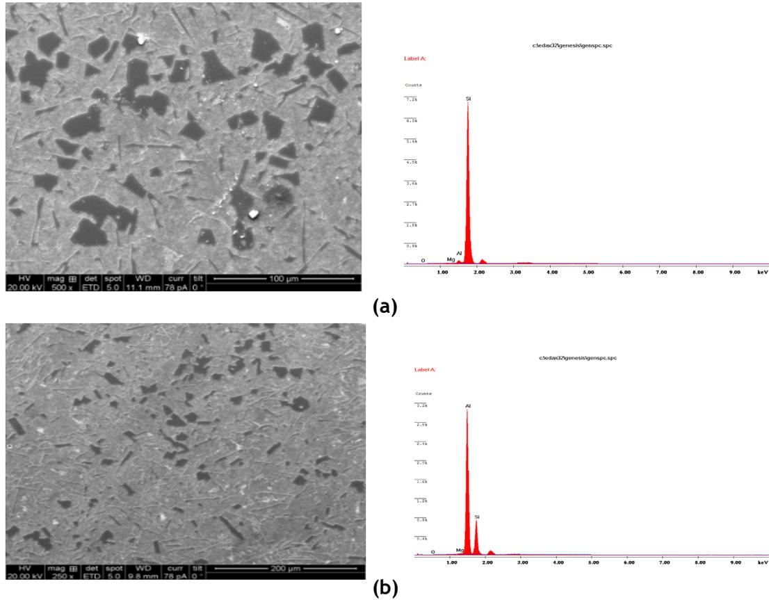
**Figure 4.** (a). SEM images of 8 mm thick castings at 800 rpm. (b). SEM images of 8 mm thick castings at 1200 rpm.
