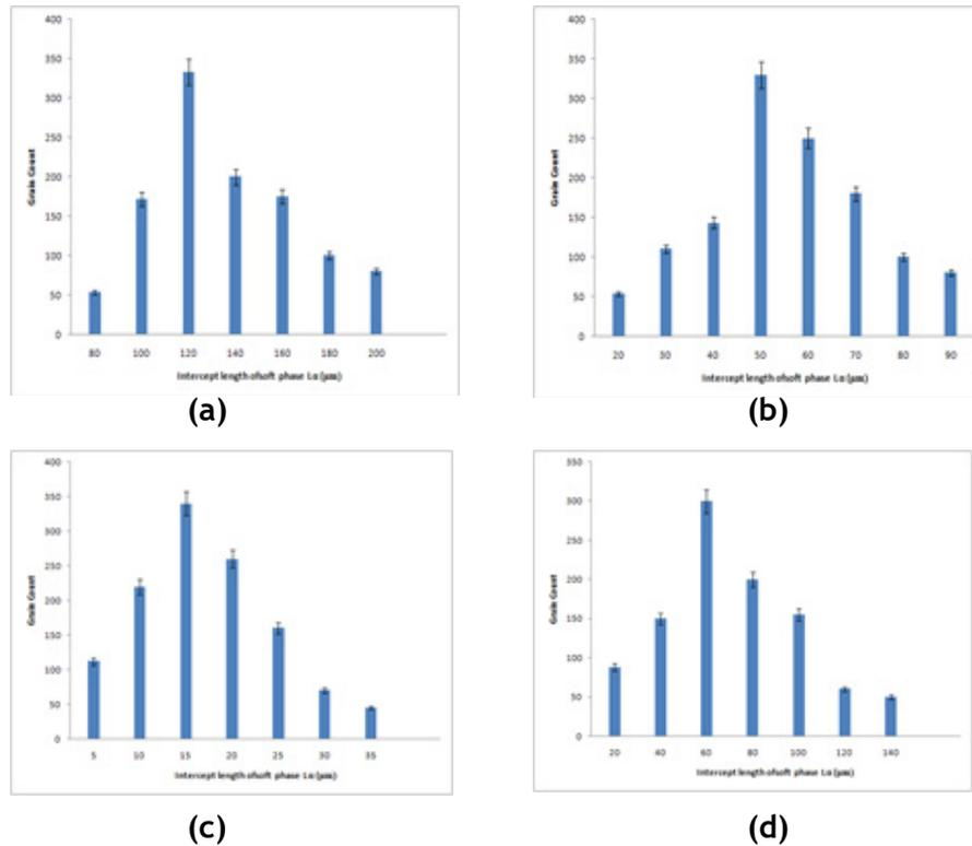
**Figure 5.** Grain count numbers v/s intercepts lengths of soft phase La (Al-17Si Alloy) for (a) 600 rpm (b) 800 rpm (c) 1000 rpm and (d) 1200 rpm (respectively from top to bottom).
