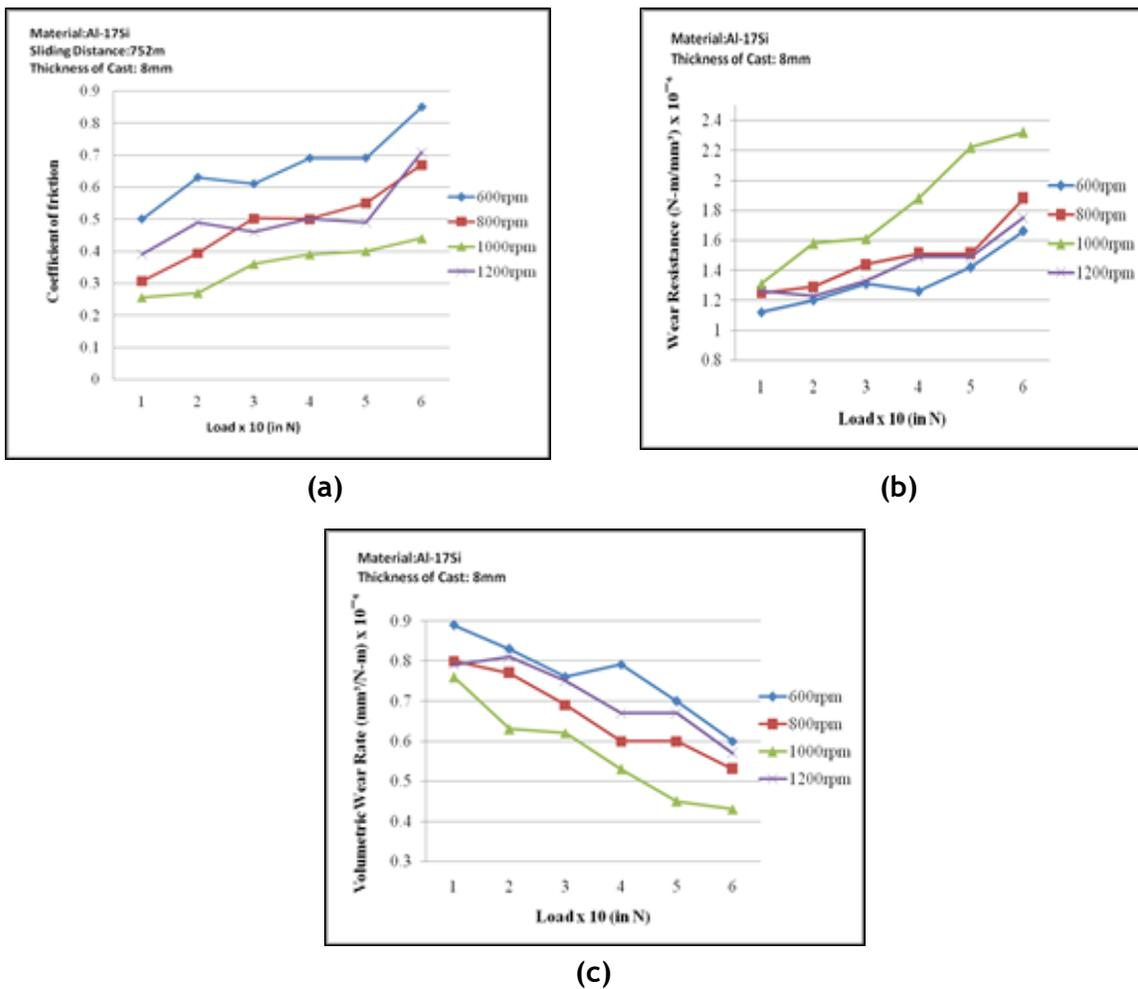
**Figure 9.** (a) Coefficient of friction v/s load. (b) Volumetric wear rate v/s load. (c) Wear resistance v/s load.
