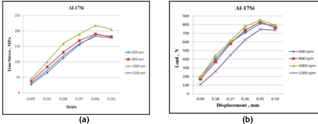
**Figure 7.** Tensile test of Al-17Si at speeds of 600, 800, 1000, and 1200 (speed units are in rpm). (a) True stress v/s Strain. (b) Load v/s Displacement
