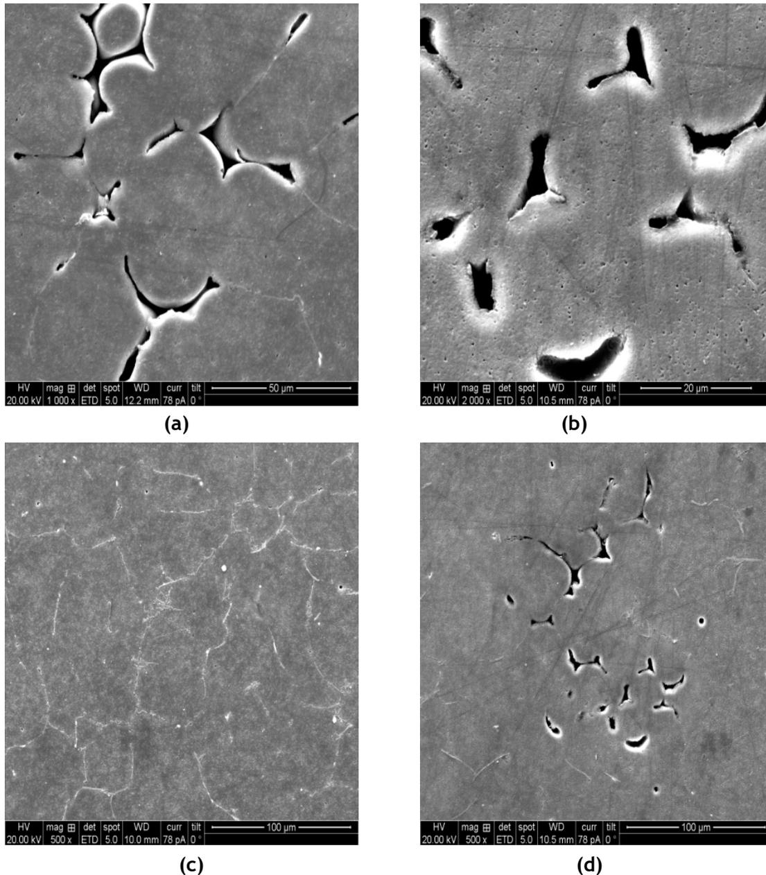
**Figure 10.** Crack growth near grain boundaries for (a) 600 rpm, (b) 800 rpm, (c) 1000 rpm and (d) 1200 rpm
