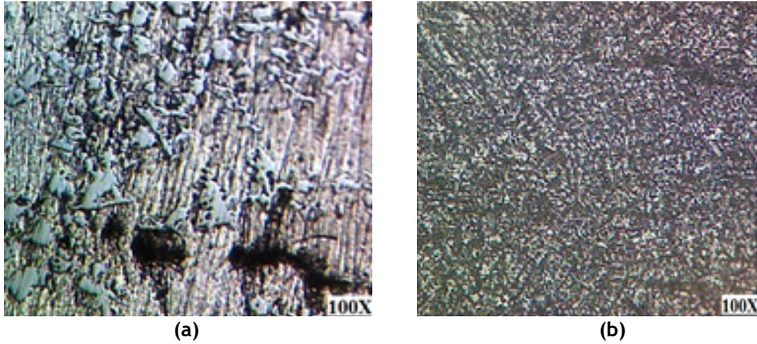
**Figure 3.** (a). Microstructure of 8mm thick Al-17Si rotated at 600 rpm. (b). Microstructure of 8mm thick Al-17Si rotated at 1000 rpm.
