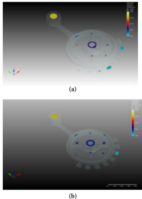
**Figure 7.** (a): Shrinkage for die temp-200°C and melt temp-700°C. (b): Shrinkage for die temp-210°C and melt temp-710°C.
