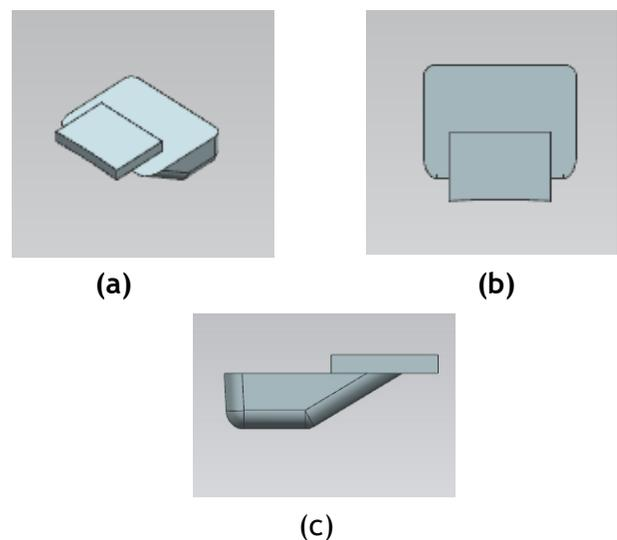
**Figure 1.** (a): Isometric view of overflows.(b): Top view of overflows. (c): Side view of overflows. Assembly of the Components
