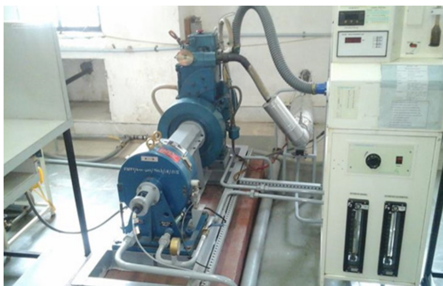
Figure 2. Photographic image of a test ring set up of a single-cylinder diesel engine.
