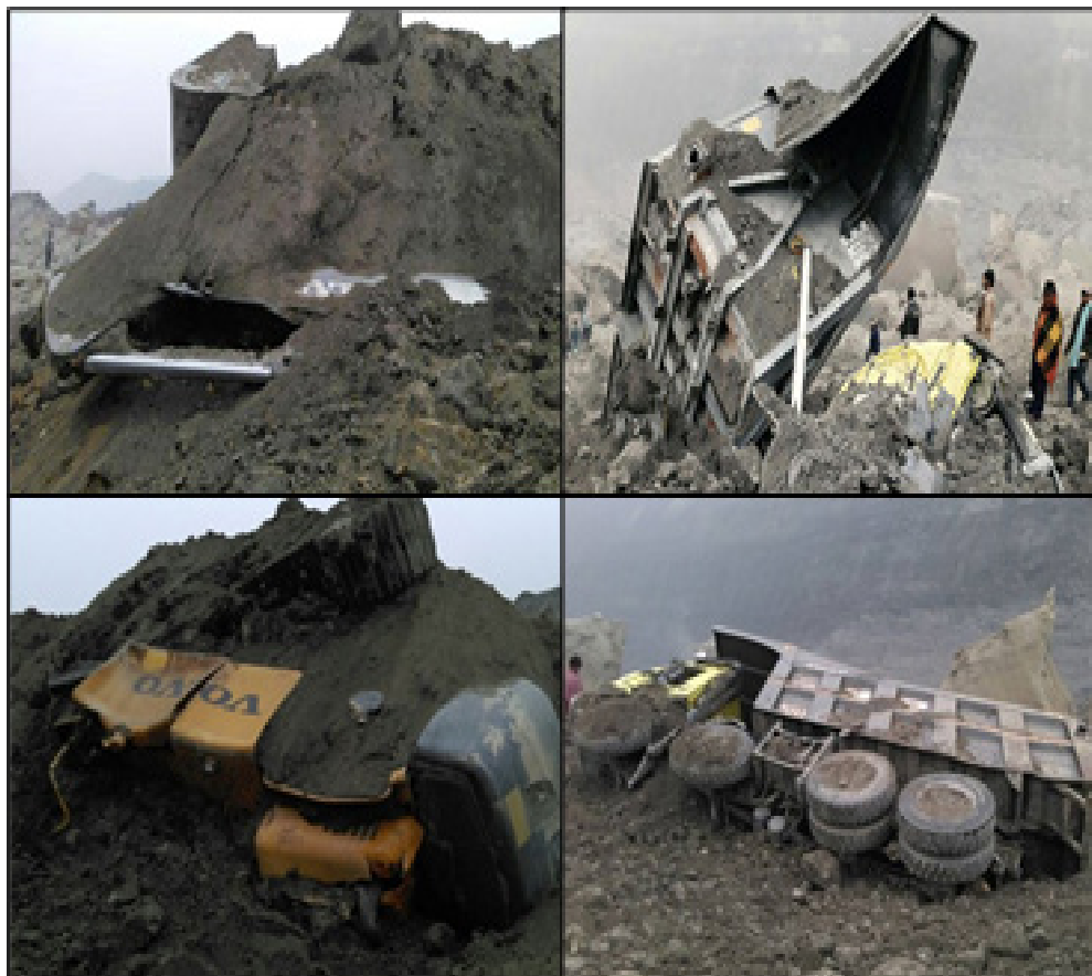
Figure 2. Mine machinery is stuck in debris flow 8 .
