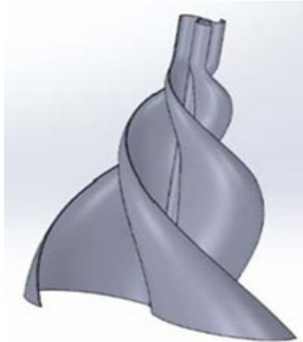
Figure 8. CAD model of nature inspired shape of VAWT blades.
