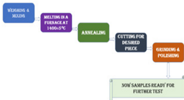
Figure 1. Flow chart of Bioglass samples prepared by the glass melting route.
