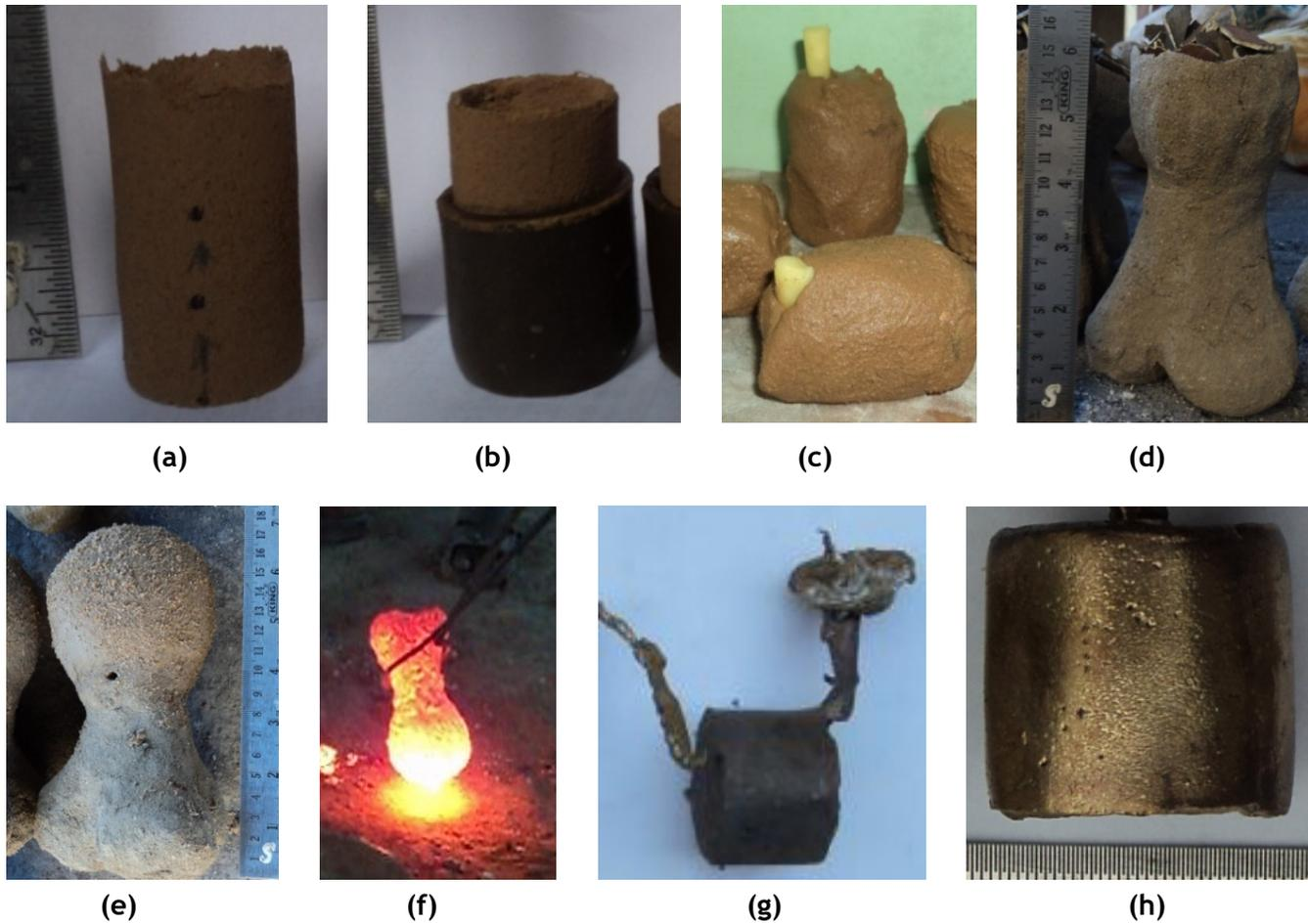
**Figure 1.** Steps of Production of Candle Stand: (a) Clay Core, (b) Wax Pattern, (c) Clay Mold (Primary Clay Coating), (d) Clay Mold (Secondary Clay) with cup; filled with brass scrap, (e) Covered clay mold, (f) Liquid metal Poured in Fired mold-pouring, (g) Cast product with gating system, (h) Cast Products.
