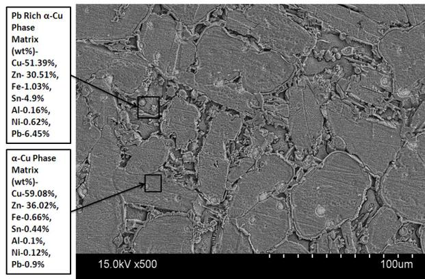
**Figure 4.** [Etchant: FeCl3 in HCL] Microstructure of Investment Casting. Developed in this design shows  $\alpha$  – Cu phase dendrites as matrix surrounded by  $\beta$  – phase. All the grains are coarse in nature indicating slow rate of cooling in hot molds.
