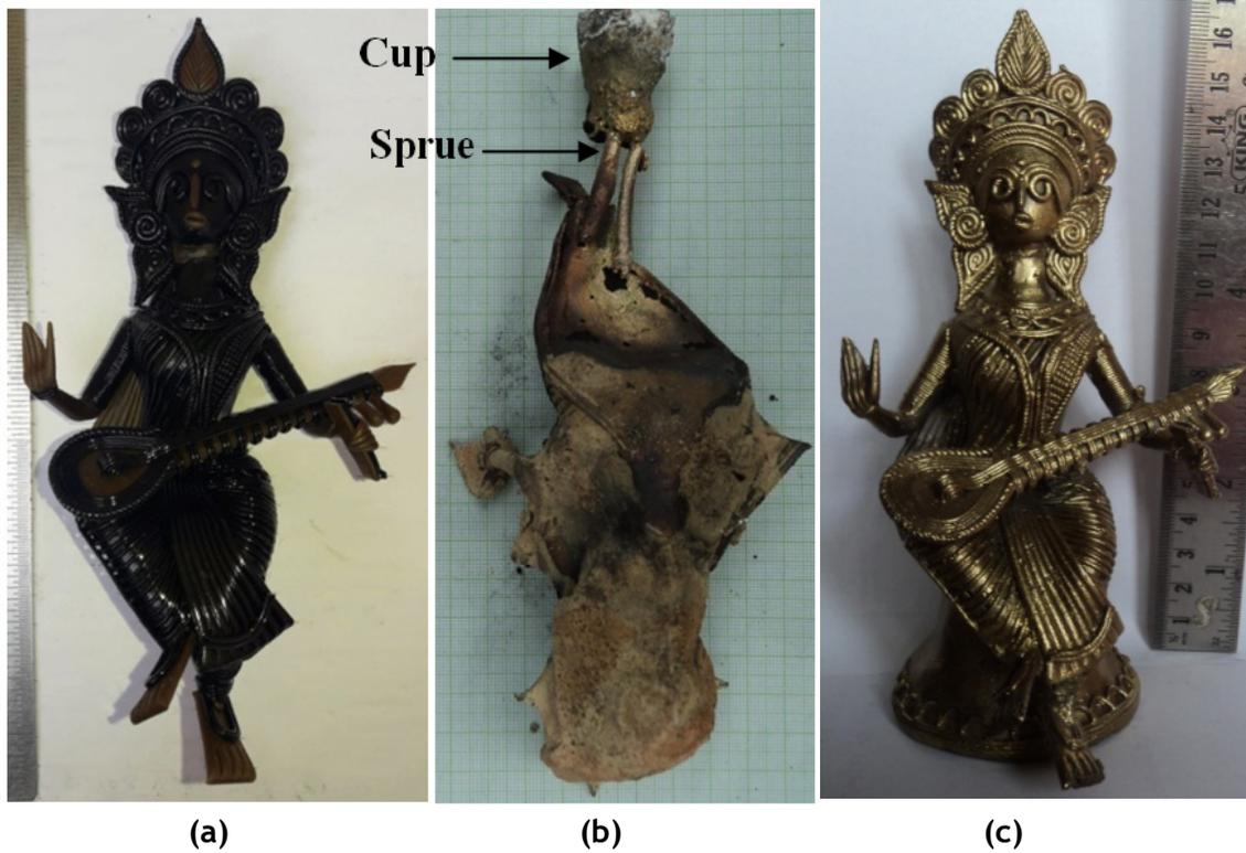
Figure 2. . (a) Wax Patten, (b) casting with gating system, (c) Finished Model.
