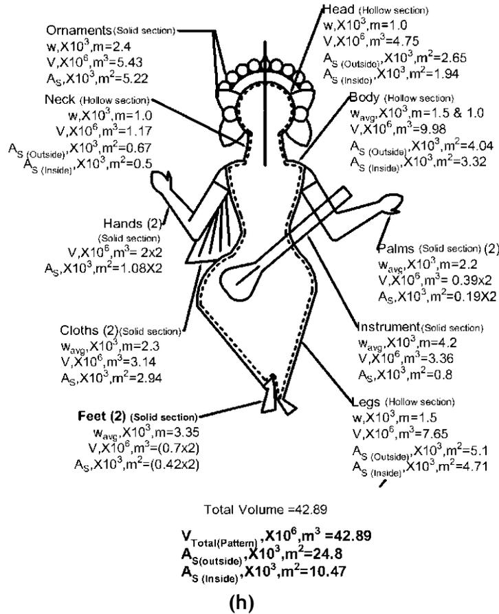
Figure 3. Schematic diagram of (a) head, neck and ornaments, (b) body, (c) hand, (d) music instrument, (e) cloths, (f) legs and feet, (g) clay mold with gating system and liquid metal flow direction, (h) overall schematic diagram of the model with volume, inside and outside surface area.
