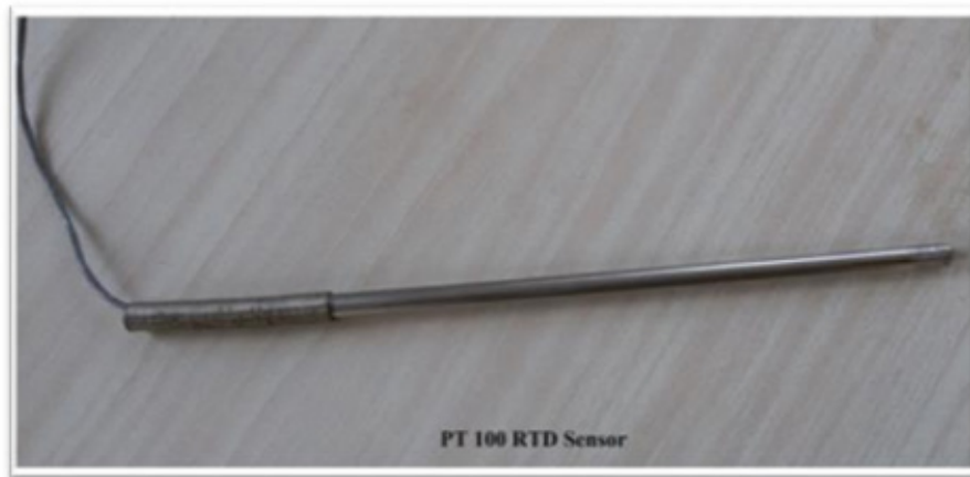
Figure 6. Photographic view of RTD Sensor.
