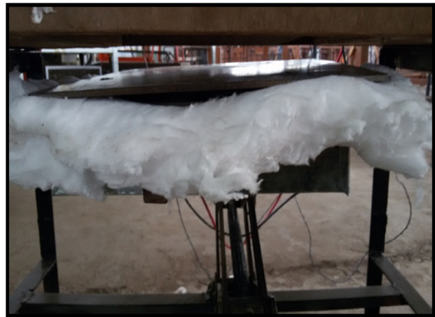
Figure 3. M. S plate electric hater of 200 W.
