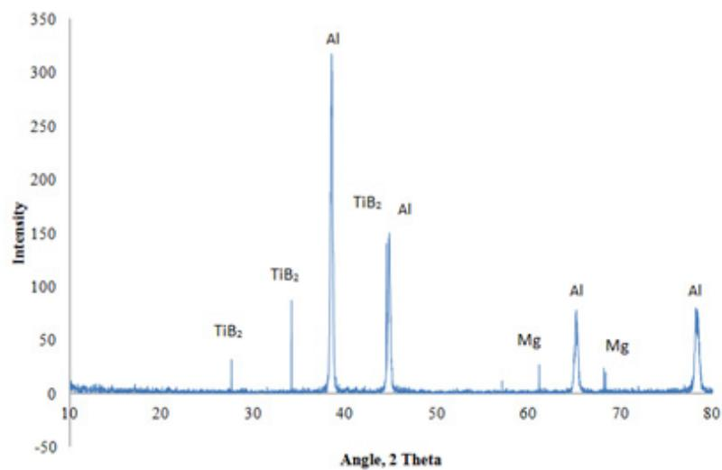
Figure 5. XRD pattern of Al6061+ 6% of  $TiB_2$ .
