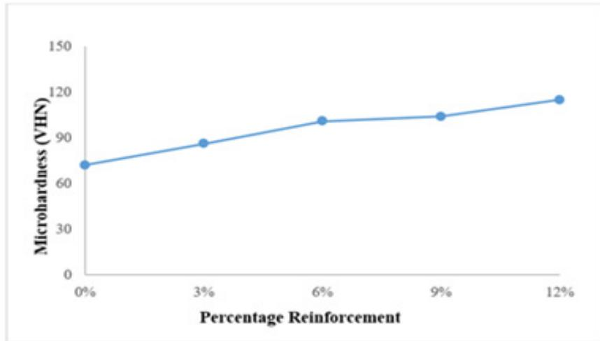
Figure 11. Micro hardness of Al6061/ TiB<sub>2</sub> composites.
