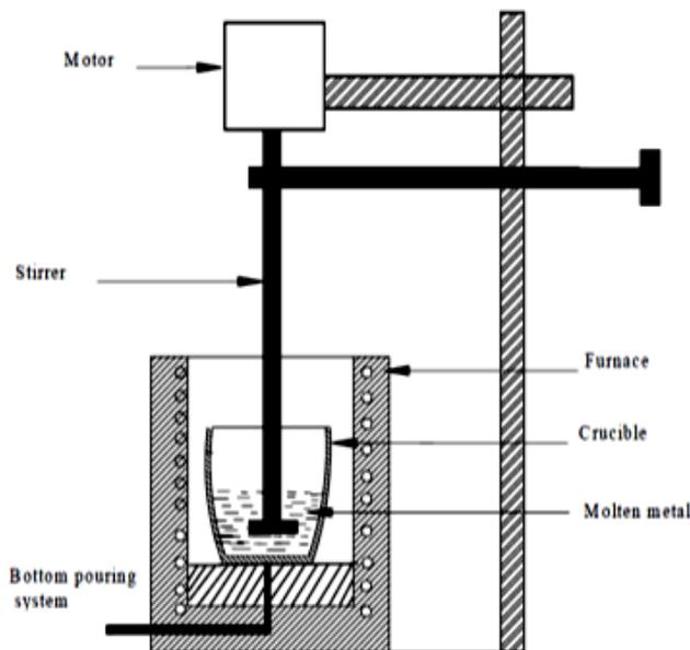
**Figure 1.** Stir casting process.
