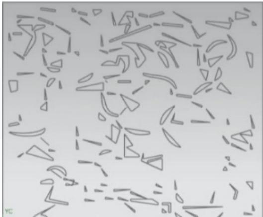
2-D drawing of microstructure
