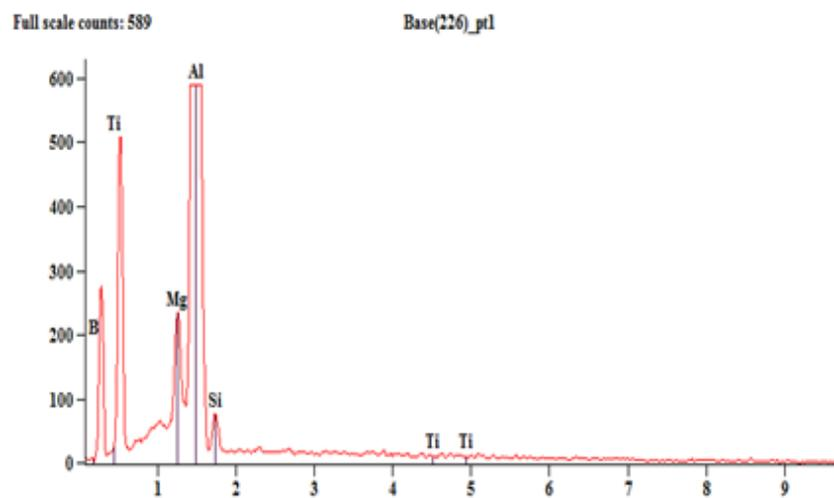
Figure 4. EDS spectrum Al6061+ 6% of  $TiB_2$ .
