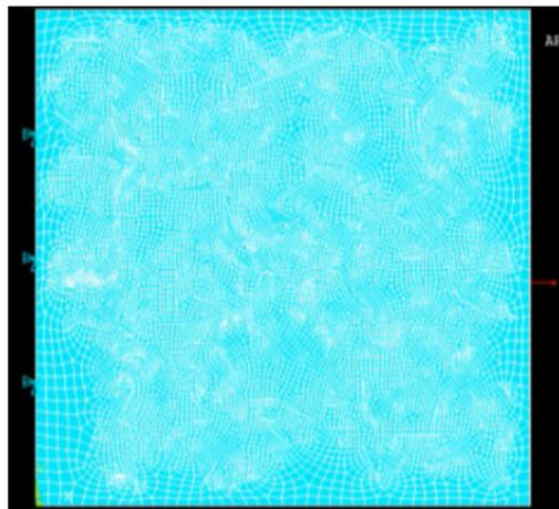
Load and displacement boundary conditions for FEA
