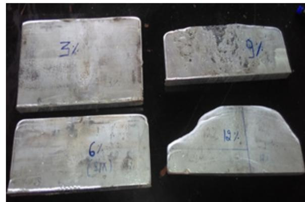
**Figure 3.** Al6061-TiB<sub>2</sub> castings.
